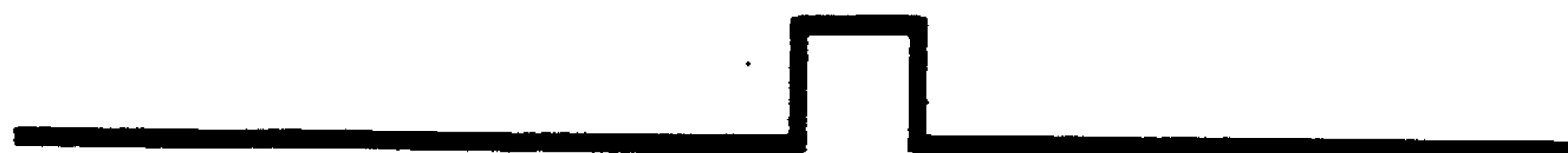
FIGURE 2C. Radio 2 Spacer Pulse for Dual De-Squelch
