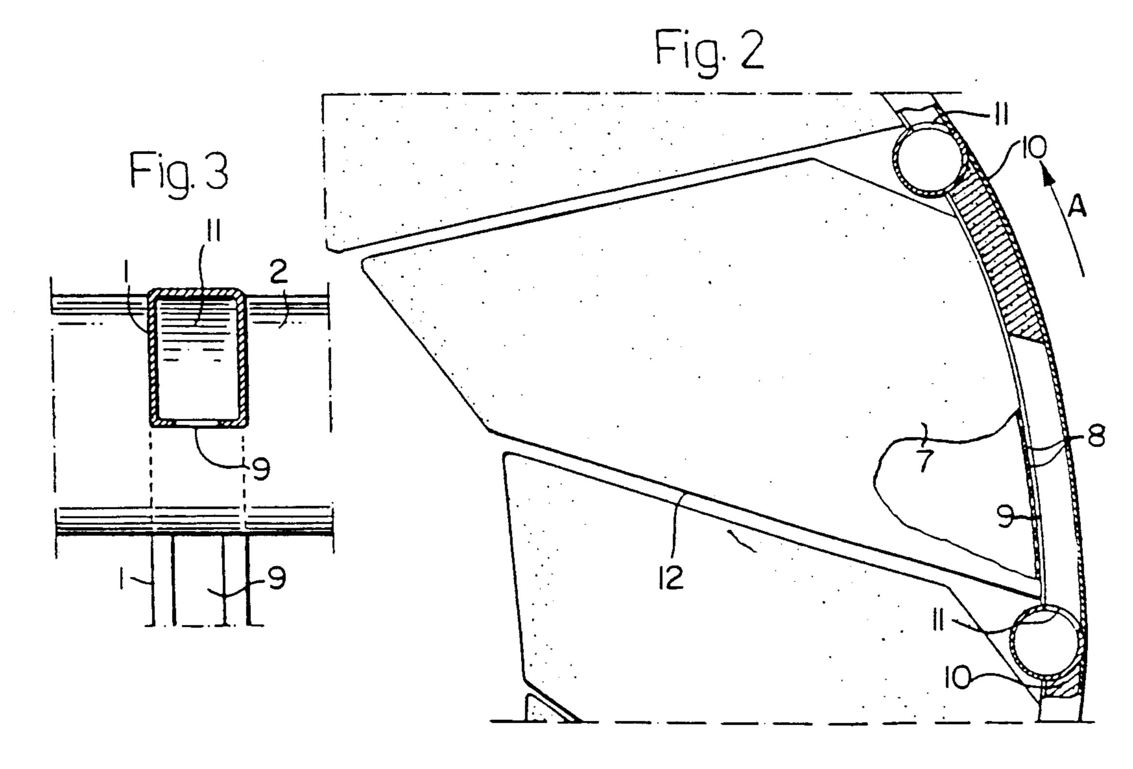
ROTATING FILTER WITH OUTER FILTRATE CONDUITS
