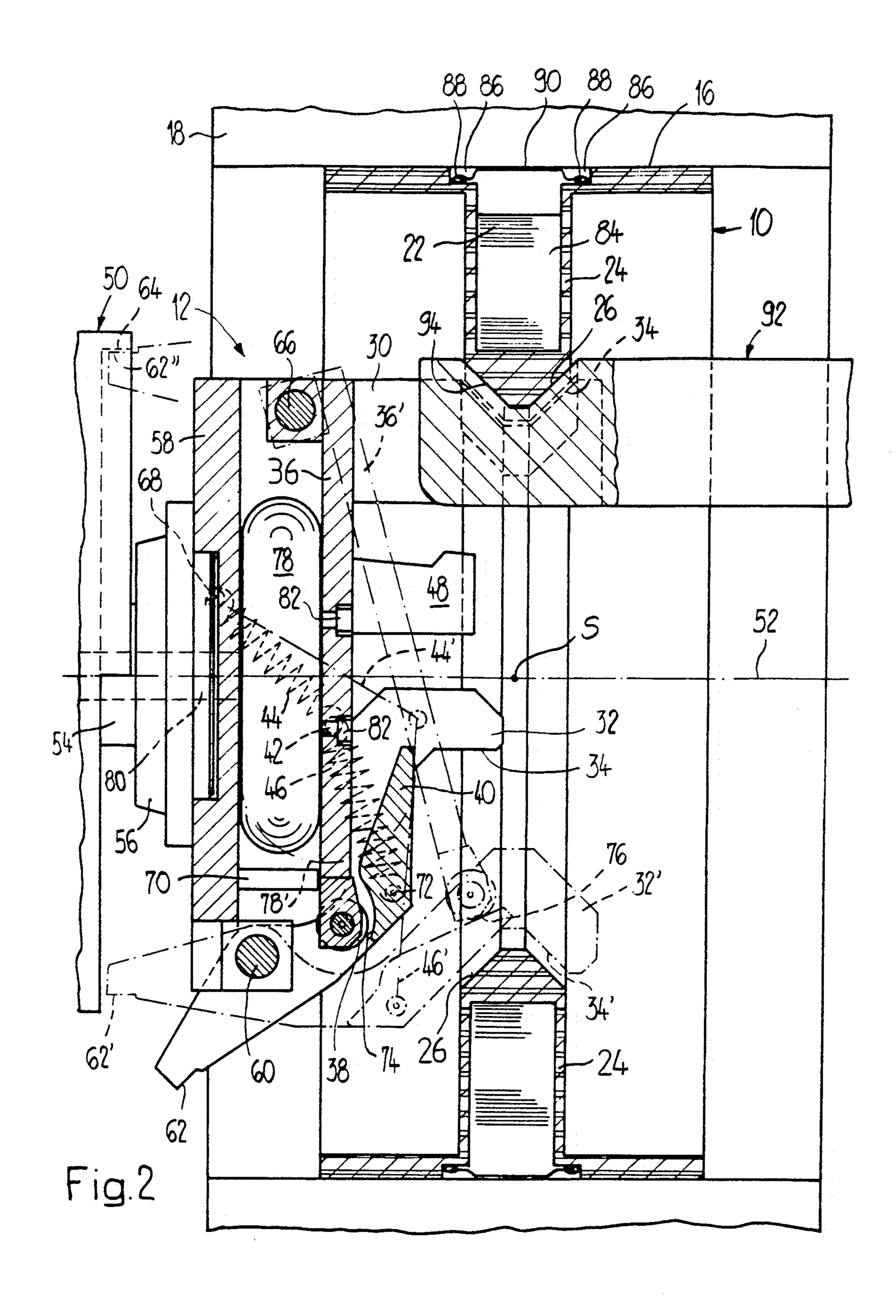
APPARATUS FOR ROTATABLY SUPPORTING A HOLLOW, SUBSTANTIALLY CYLINDRICAL WINDING CORE, AND WINDING CORE FOR SUPPORTING A COIL OF FLEXIBLE, SUBSTANTIALLY FLAT PRODUCTS, ESPECIALLY PRINTED PRODUCTS
