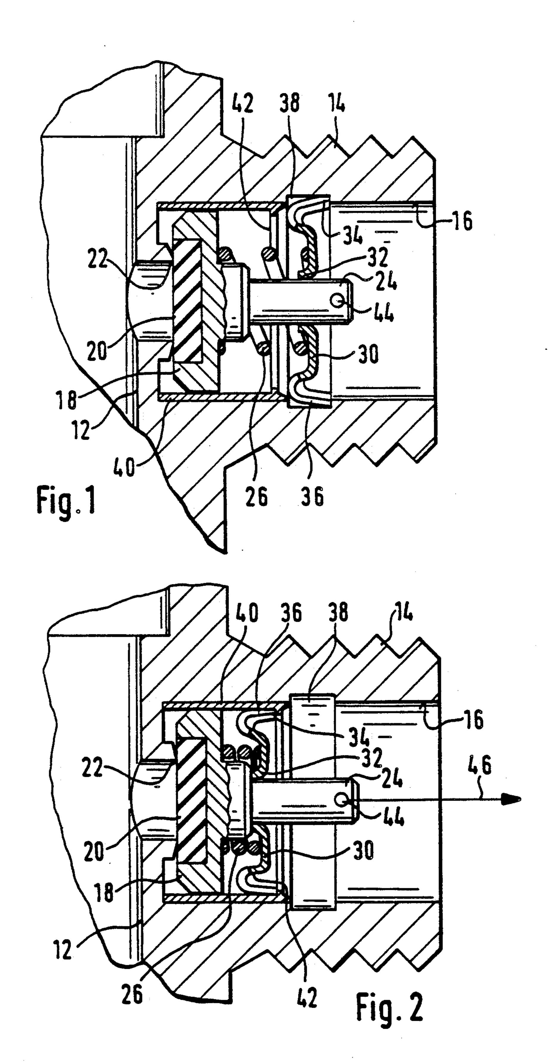
is urged elastically and radially outwards so as to rest either on the edge of an inner circular groove of the said bore, in order to keep the valve in the operative position, or, under the action of a manual depression, behind
