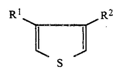
wherein R<sup>1</sup> and R<sup>2</sup> are certain specified substituent groups can be homopolymerized or copolymerized to form polymers which are electroconductive. These polymers find many uses, for example, as EMI/RF shielding materials, in electrochromic display systems, as antistatics, as ion and pH sensors, as battery electrode materials etc.
