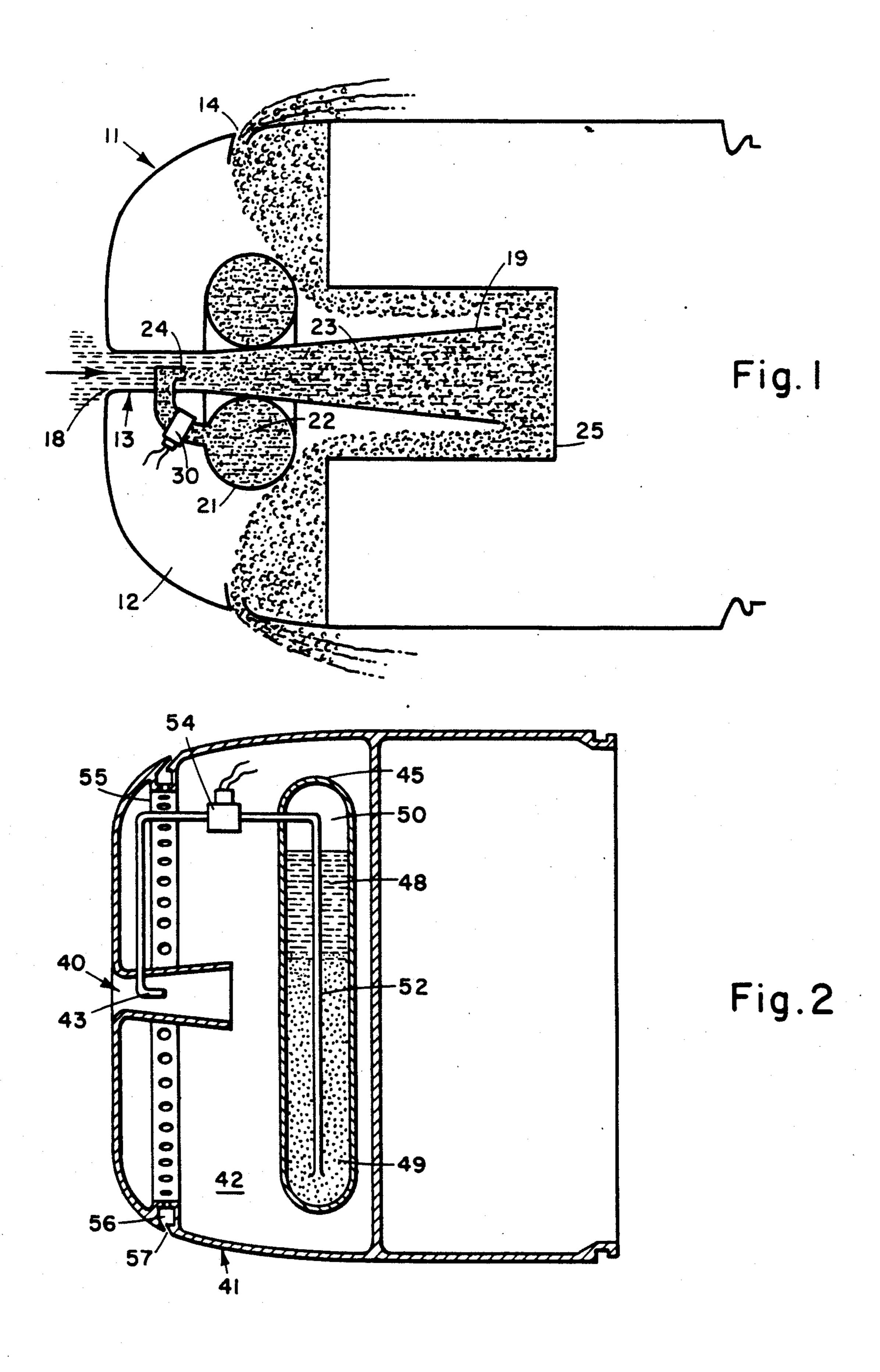
gas mixture into the boundary layer of underwater vehicles wherein the gas mixture is obtained from a powder
