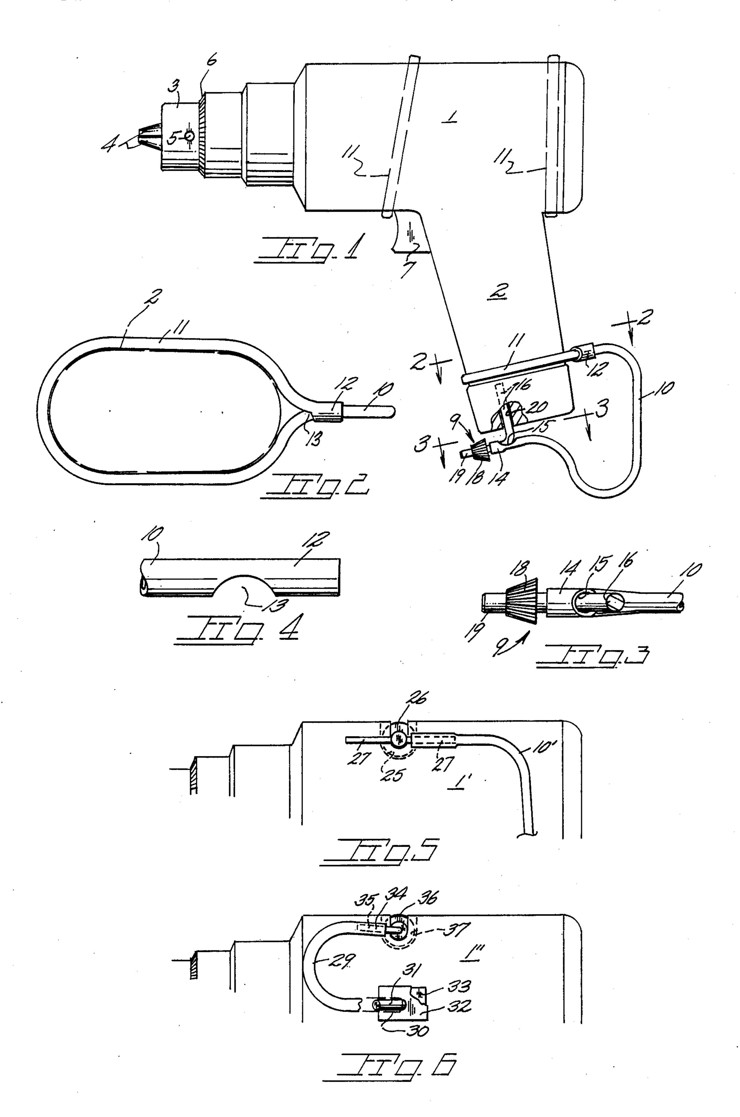
securement to a drill motor housing with the key unencumbered to enable key handled or key gear insertion
