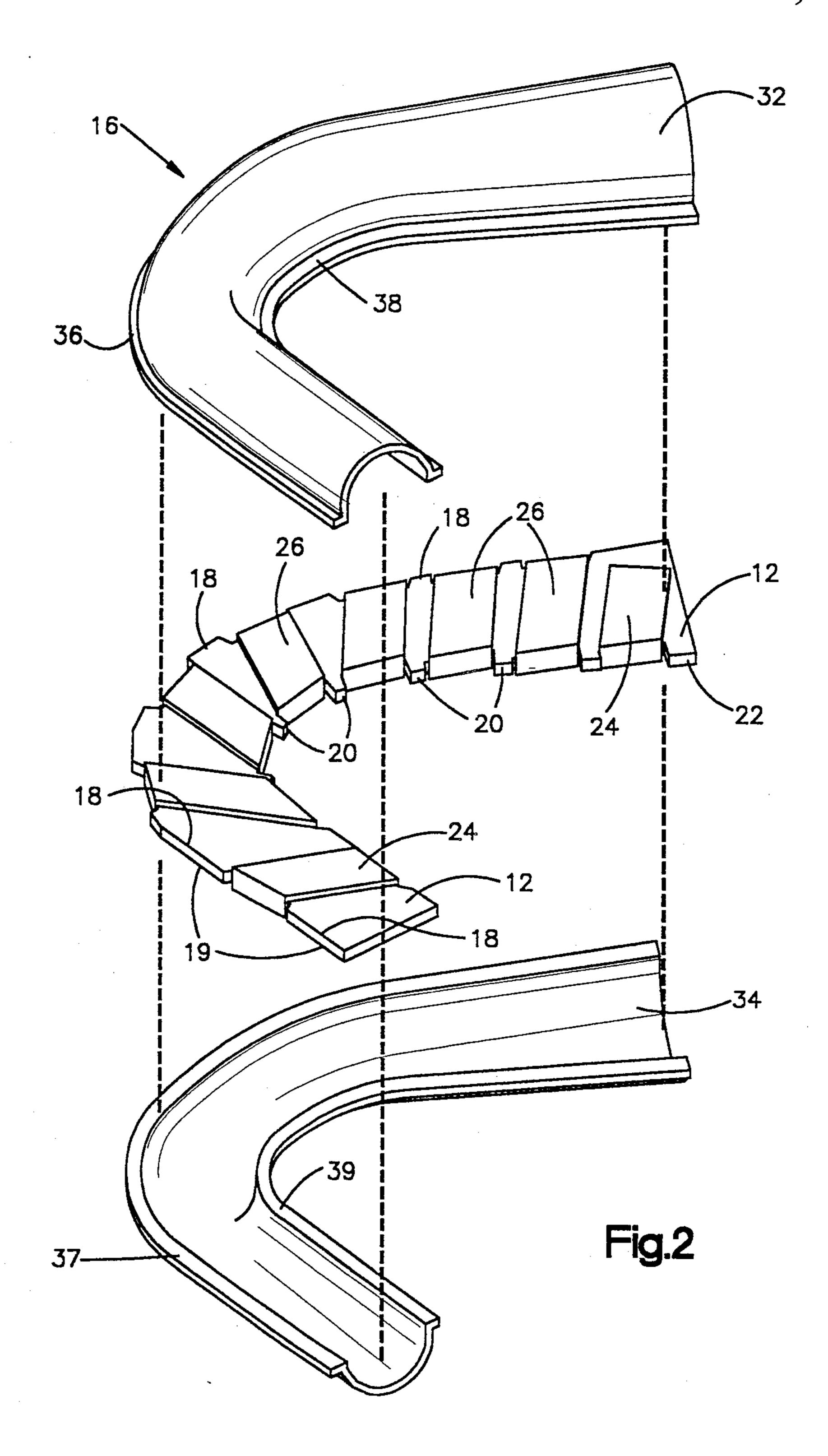
CATALYTIC EXHAUST PIPE INSERT
