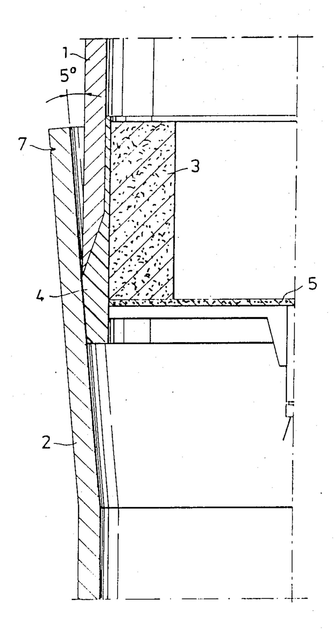
EXPLOSION-WELDED PIPE JOINT
