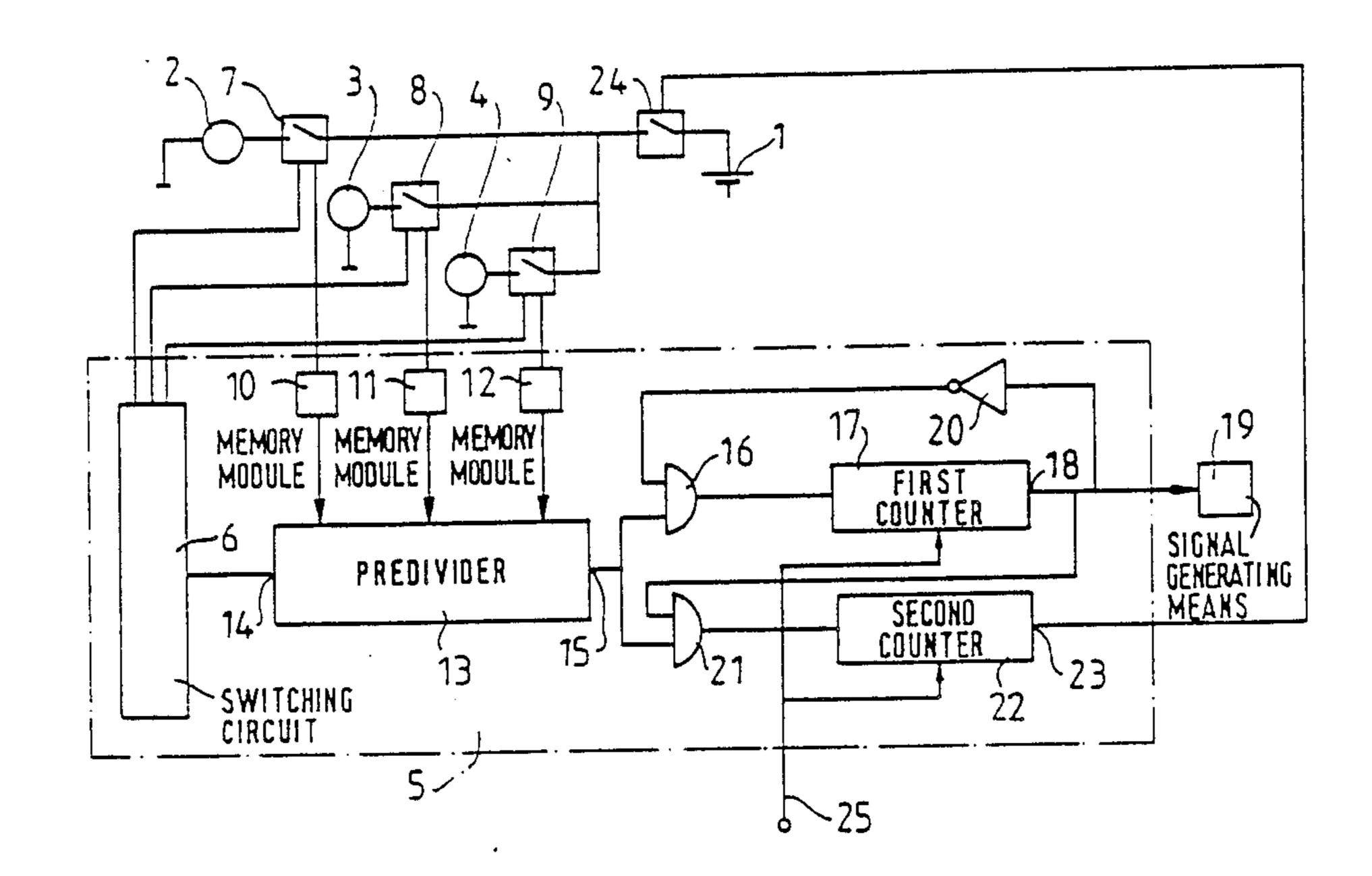
METHOD AND APPARATUS FOR MONITORING THE CONDITION OF CHARGE OF A BATTERY CONNECTED TO AN APPLIANCE AND INCLUDING COUNTERS COUNTED WITH RESPECT TO THE TIME AND DRAIN OF THE BATTERY
