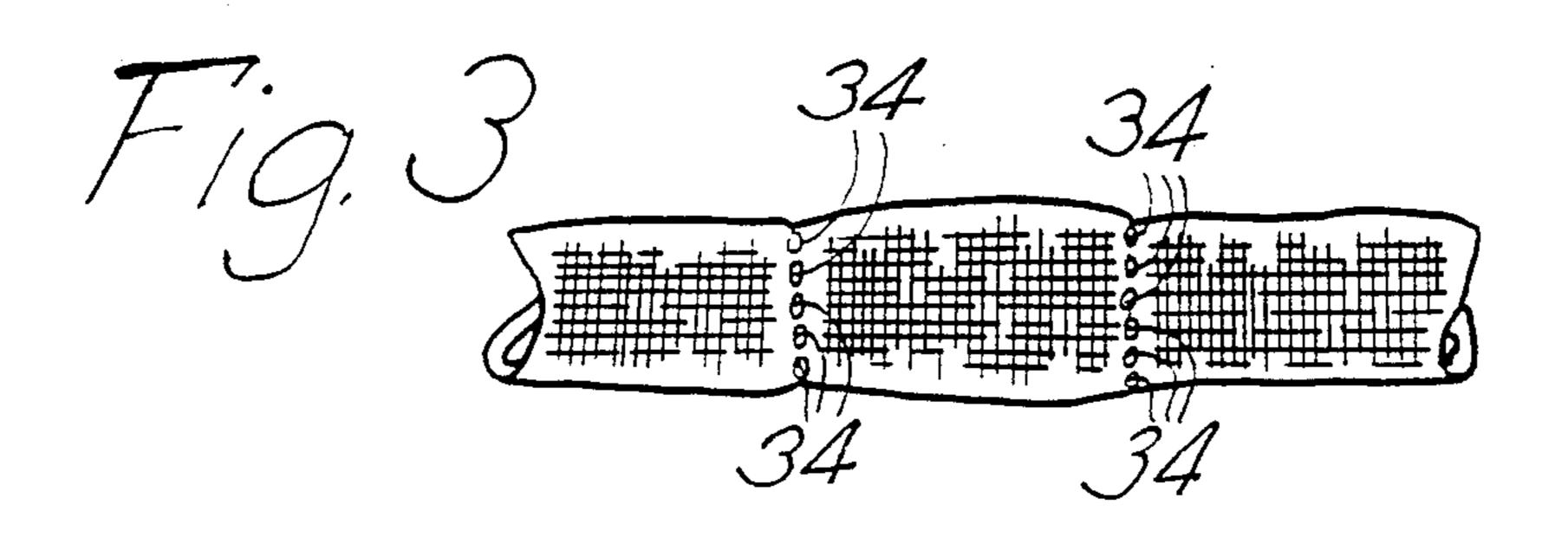
severing the tube at selected ones of the relatively short sections.
