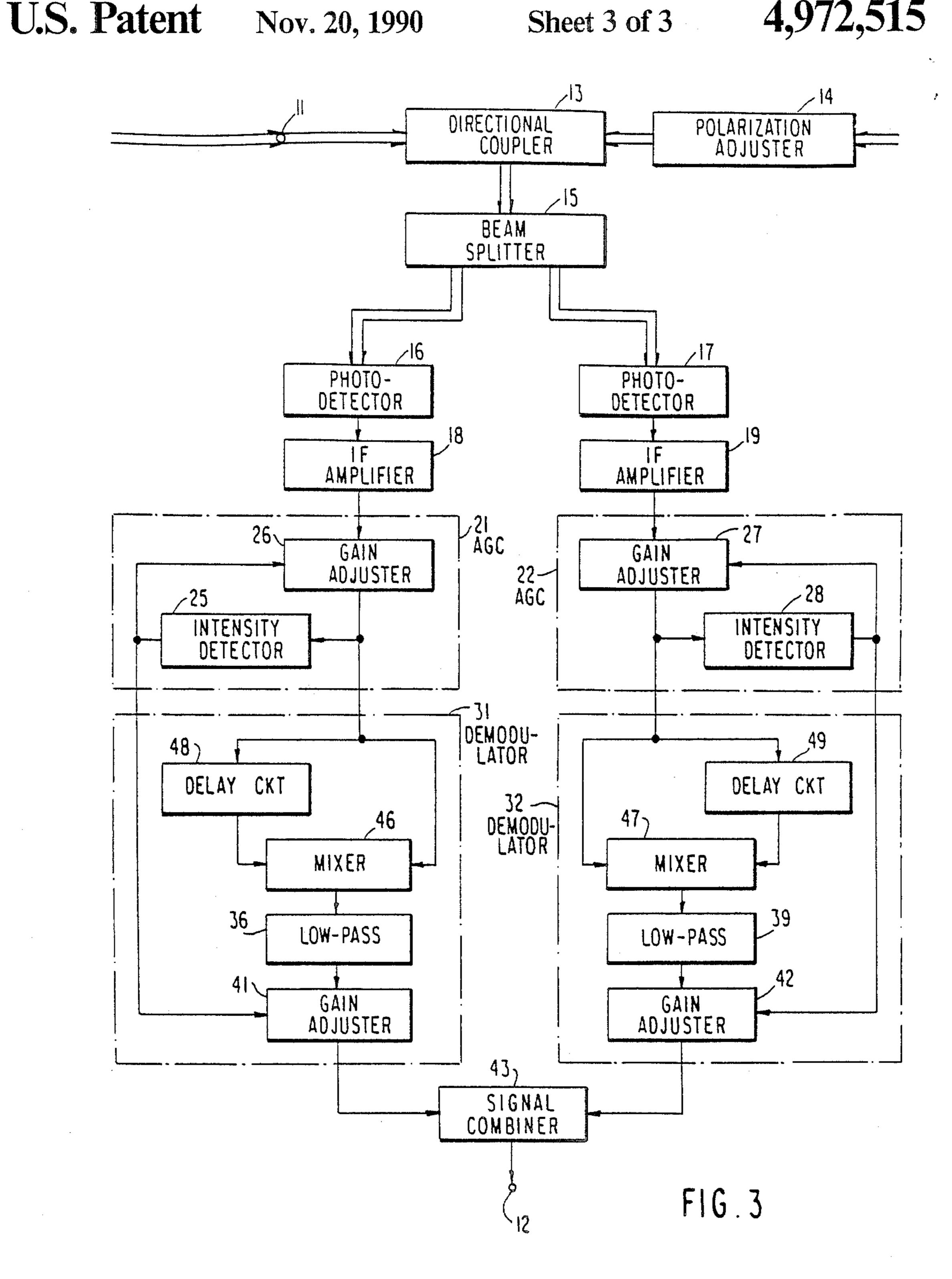
POLARIZATION DIVERSITY RECEIVER HAVING LITTLE DETERIORATED SENSITIVITY DESPITE USE OF A SQUARE-LAW DEMODULATOR HAVING A RESTRICTED DYNAMIC RANGE
