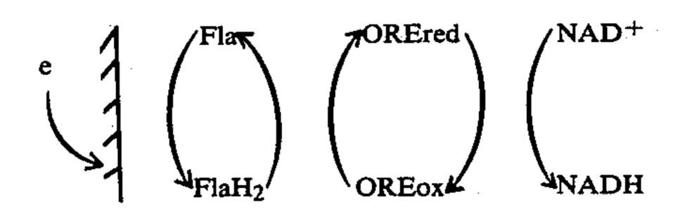
When the reduction of NAD+is carried out with FlaH<sub>2</sub>, it is necessary to have a solution containing a high concentration of FlaH<sub>2</sub> in the medium. The following process is then carried out:
