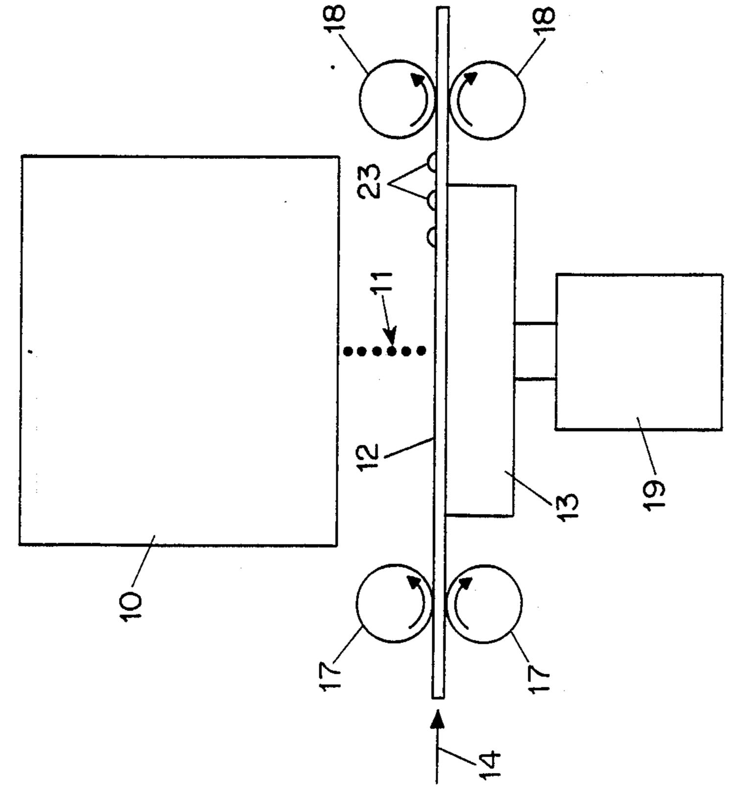
FIG. 1 is a schematic diagram showing a typical arrangement for printing hot melt ink images on porous substrates in accordance with the invention; and
