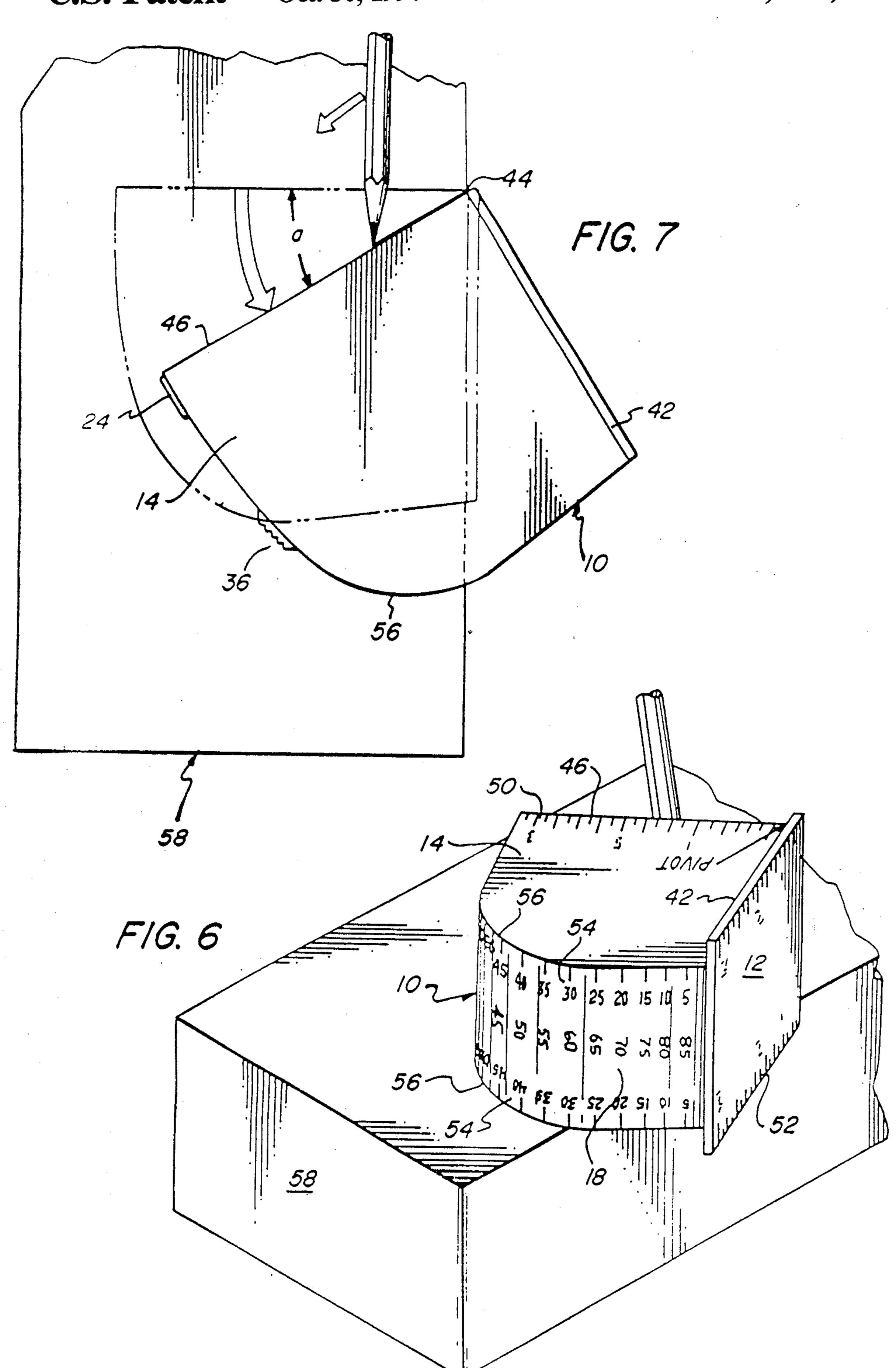
permit angular measurements to be made using the angular scale provided.
