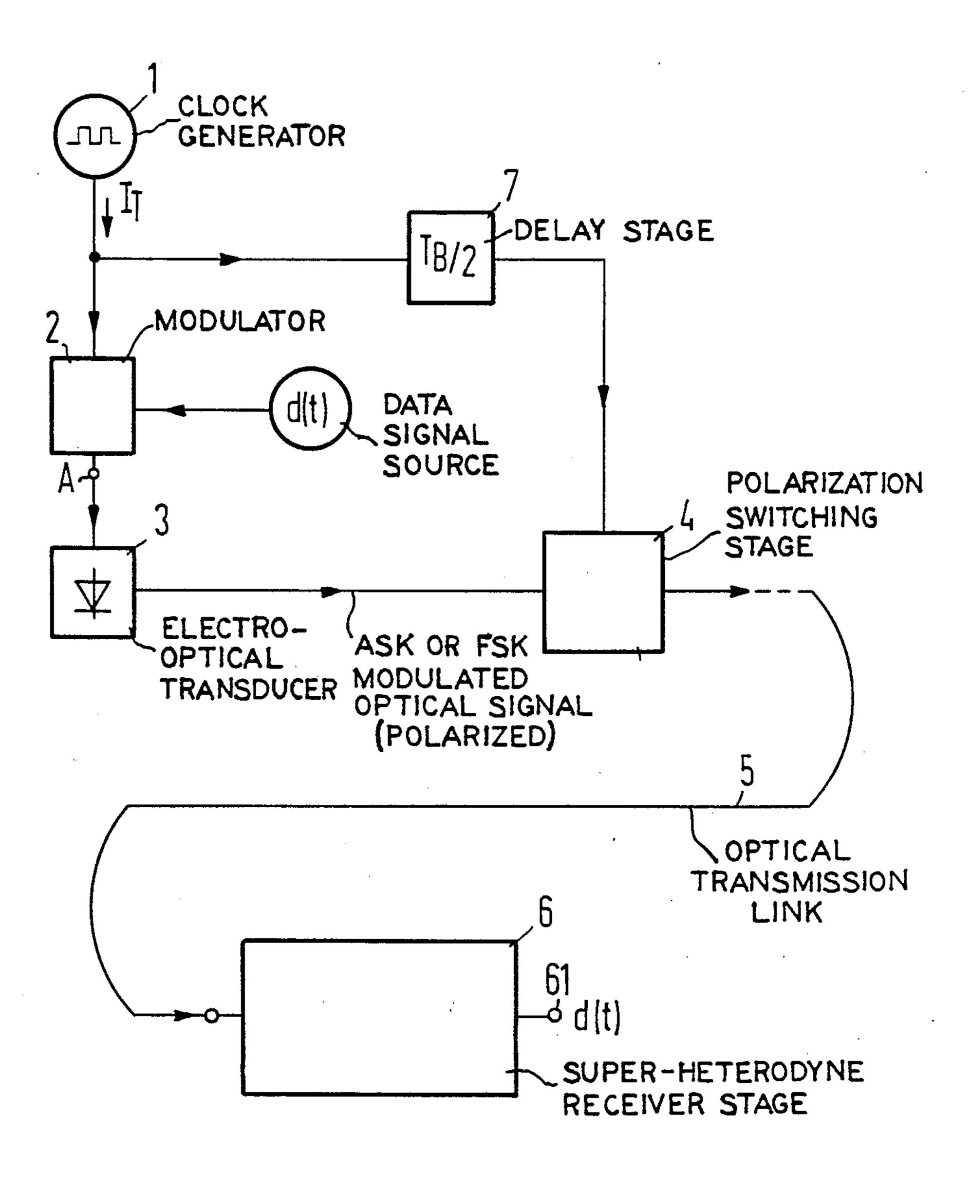
iod of the data signal. Moreover the switching signal is usually not synchronized with the data signal. METHOD FOR SYNCHRONIZED Prior art optical systems exhibit a dependency on POLARIZATION SWITCHING OF AN OPTICAL polarization which yields poor transmission quality. TRANSMISSION SIGNAL OF AN OPTICAL TRANSMISSION SYSTEM HAVING SUPERHETERODYNE RECEPTION AND AN
