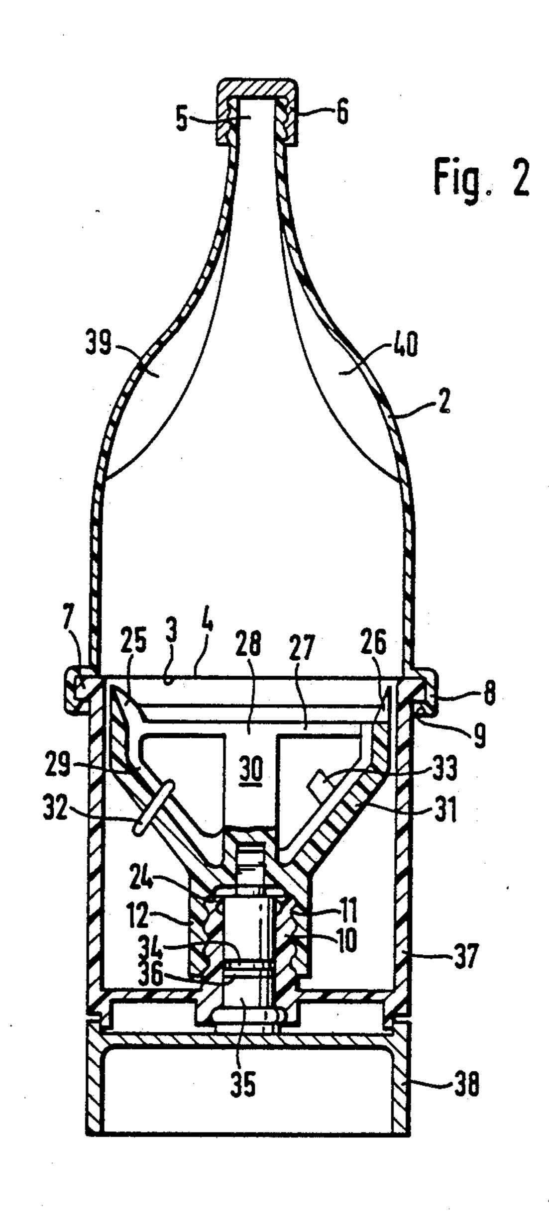
that the activating device comprises an annular portion which partially encloses the first container portion and is constructed as an upright ring.
