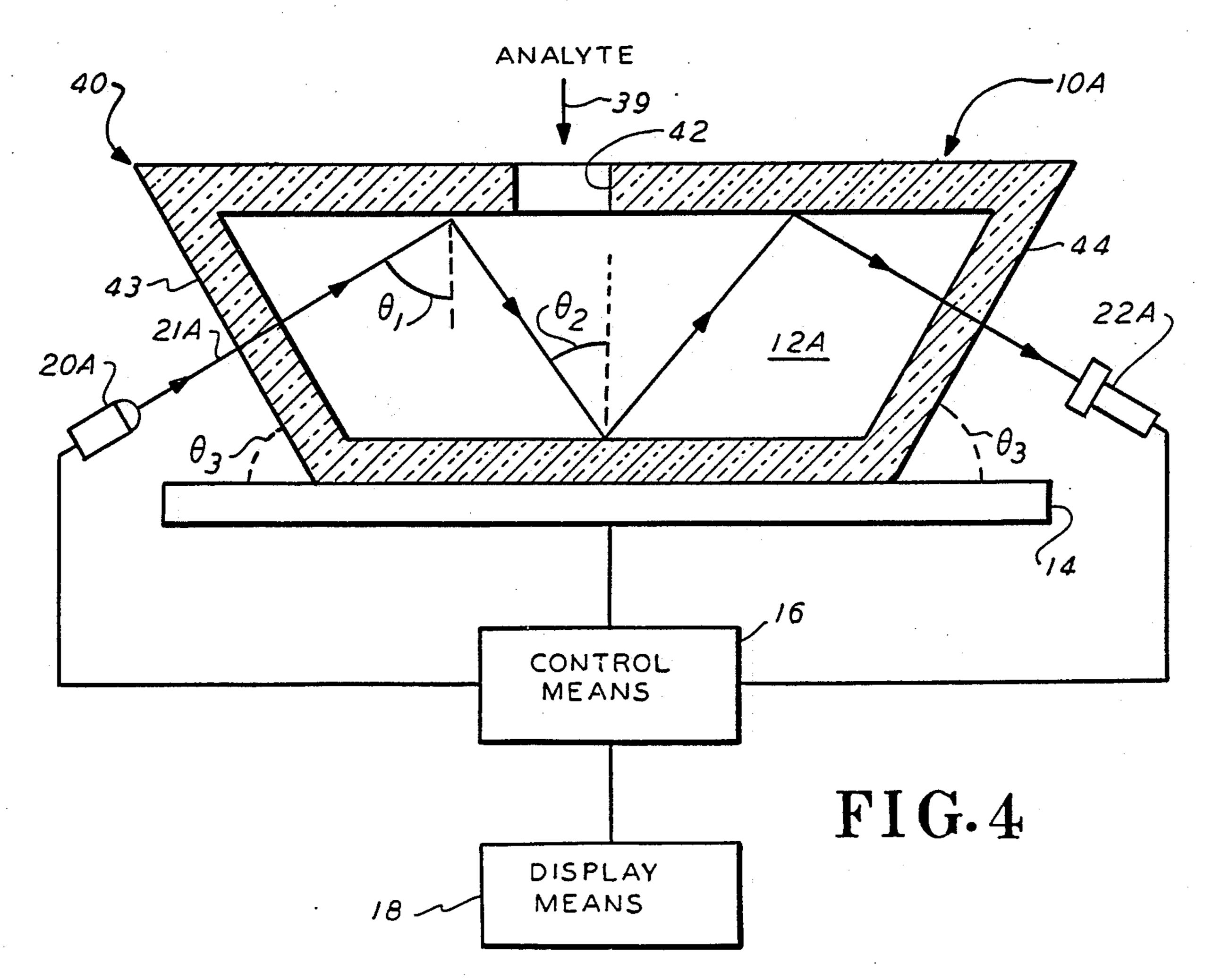
ANALYTE DETERMINATION USING GEL INCLUDING A REAGENT SYSTEM REACTS WITH ANALYTE TO CHANGE TRANSMISSIVE PROPERTY OF GEL DETECTABLE BY LIGHT BEAM TRANSMITTED THROUGH GEL BY TOTAL INTERNAL REFLECTANCE
