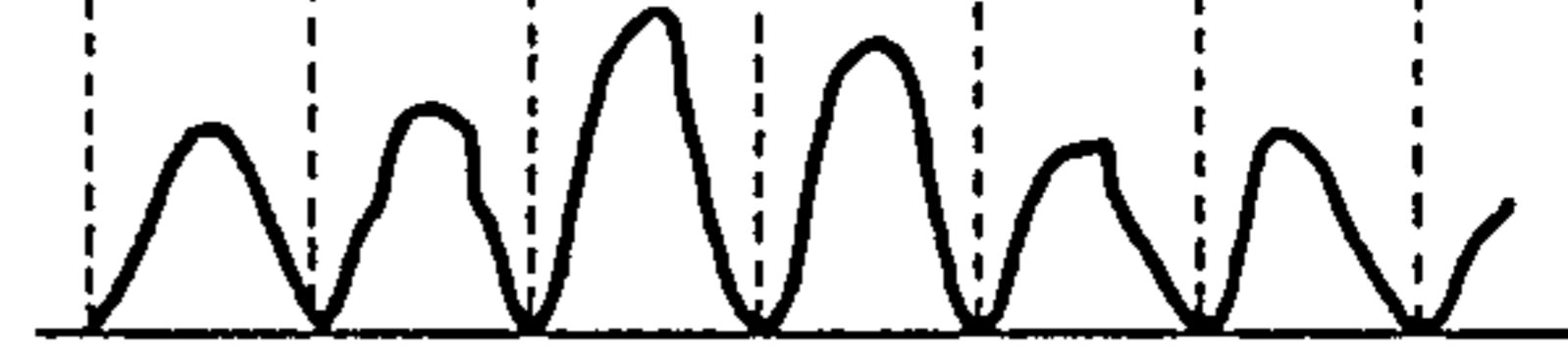
FIG. 6 (B) OUTPUT OF SQUARE CIRCUIT
