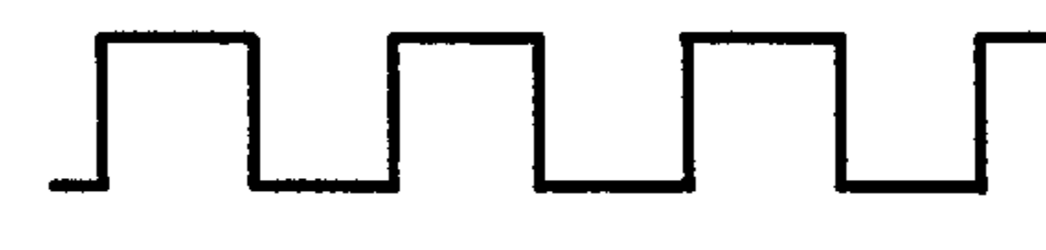
FIG. 6 (F) OUTPUT OF ONE-HALF FREQUENCY DIVIDER
