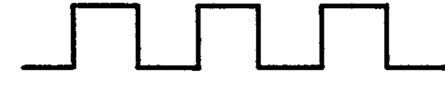
FIG. 6 (G) OUTPUT OF ONE-HALF FREQUENCY DIVIDER
