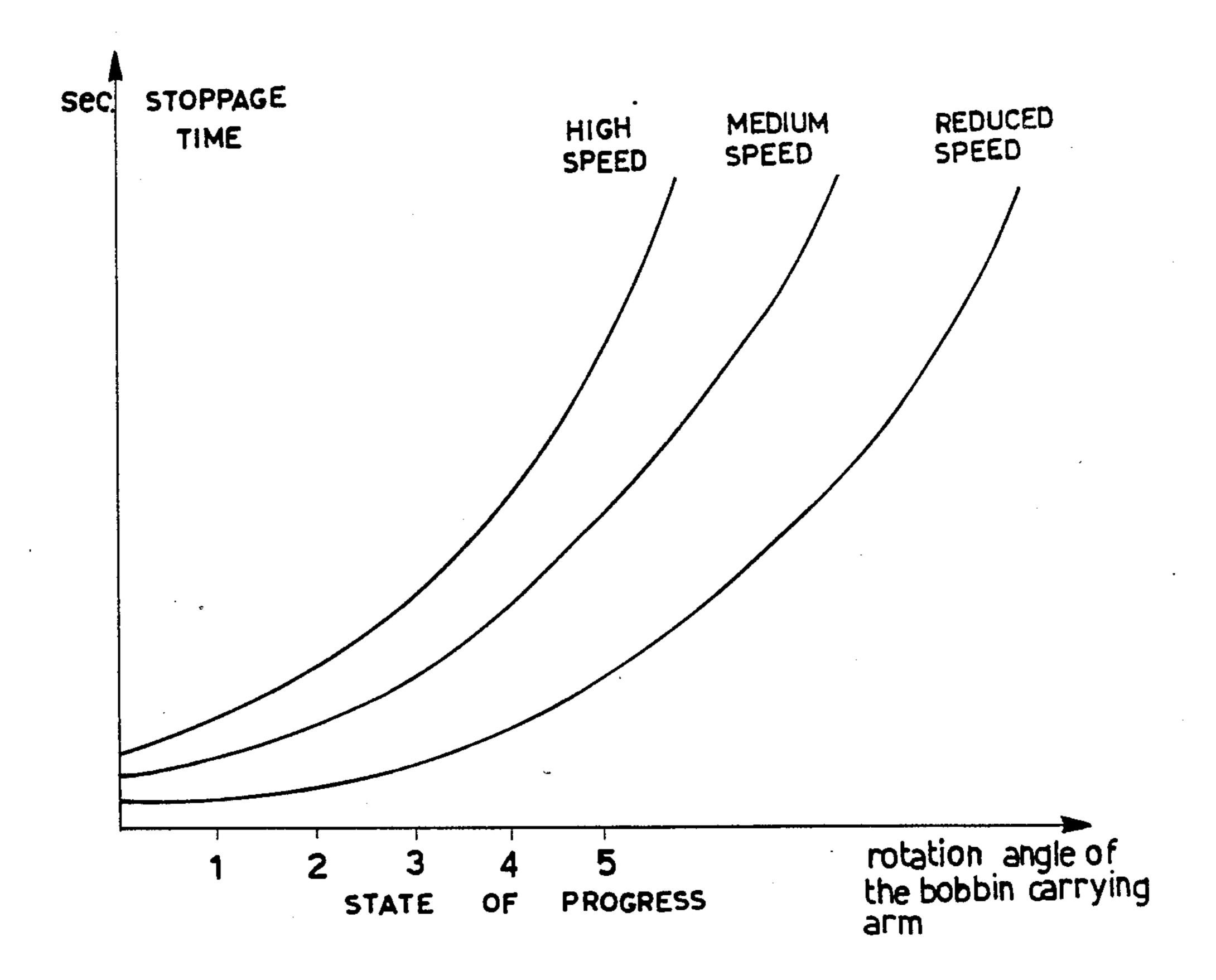
DEVELOPMENT OF BOBBIN STOPPAGE TIMES AT DIFFERENT WINDING SPEEDS AS A FUNCTION OF THE ROTATION ANGLE OF THE BOBBIN CARRYING ARM
