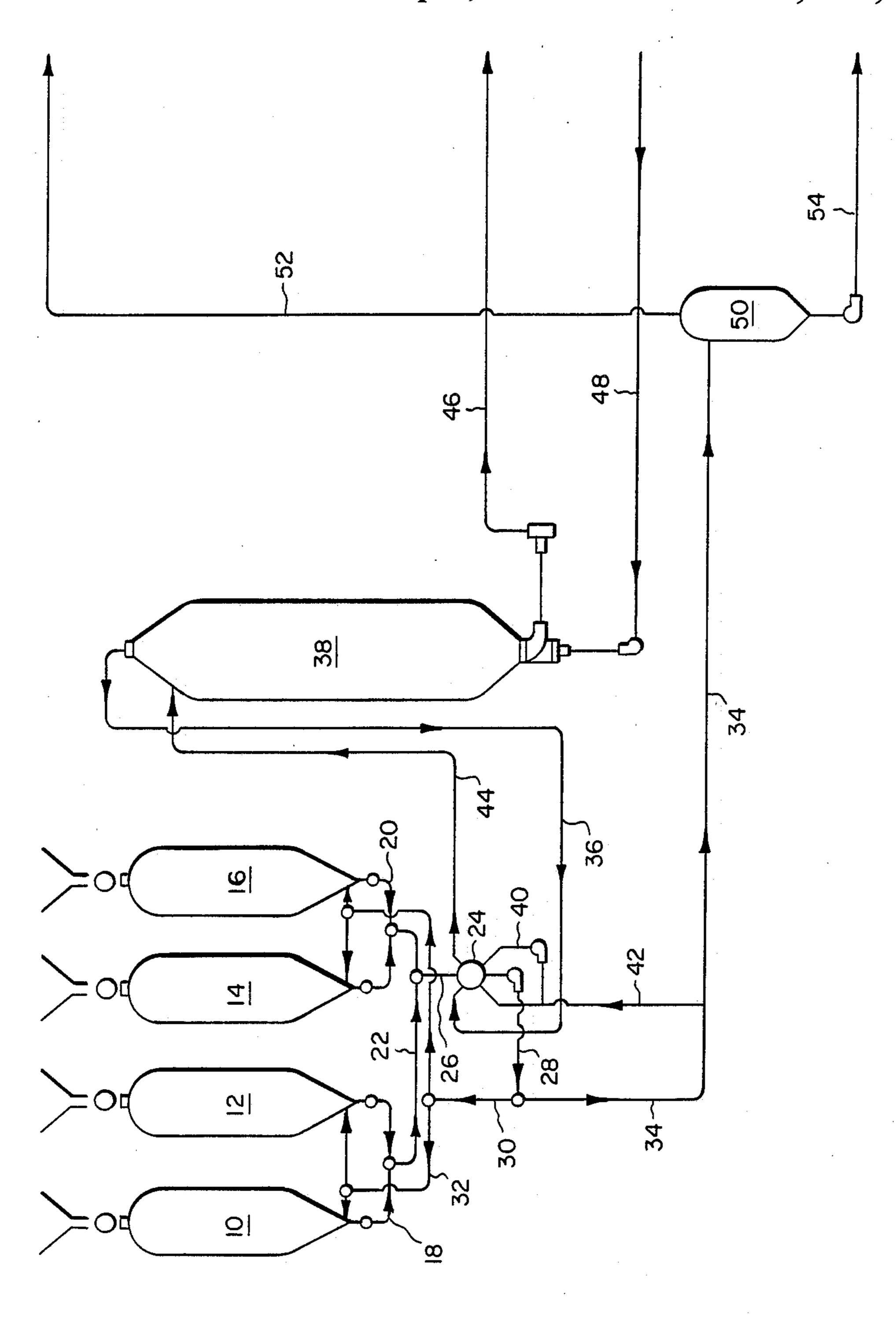
METHOD FOR TRANSFERE OF FIRROUS MATERIALS TRANSPORT BY LIQUIDS
