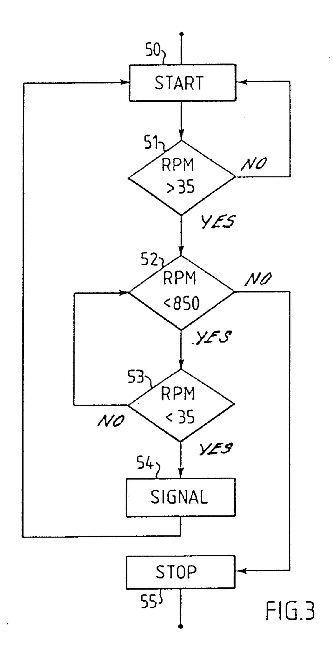
METHOD AND ARRANGEMENT FOR IMPROVING THE STARTING ABILITY OF AN INTERNAL COMBUSTION ENGINE, WHEN AN ATTEMPT TO START THE ENGINE HAS FAILED
