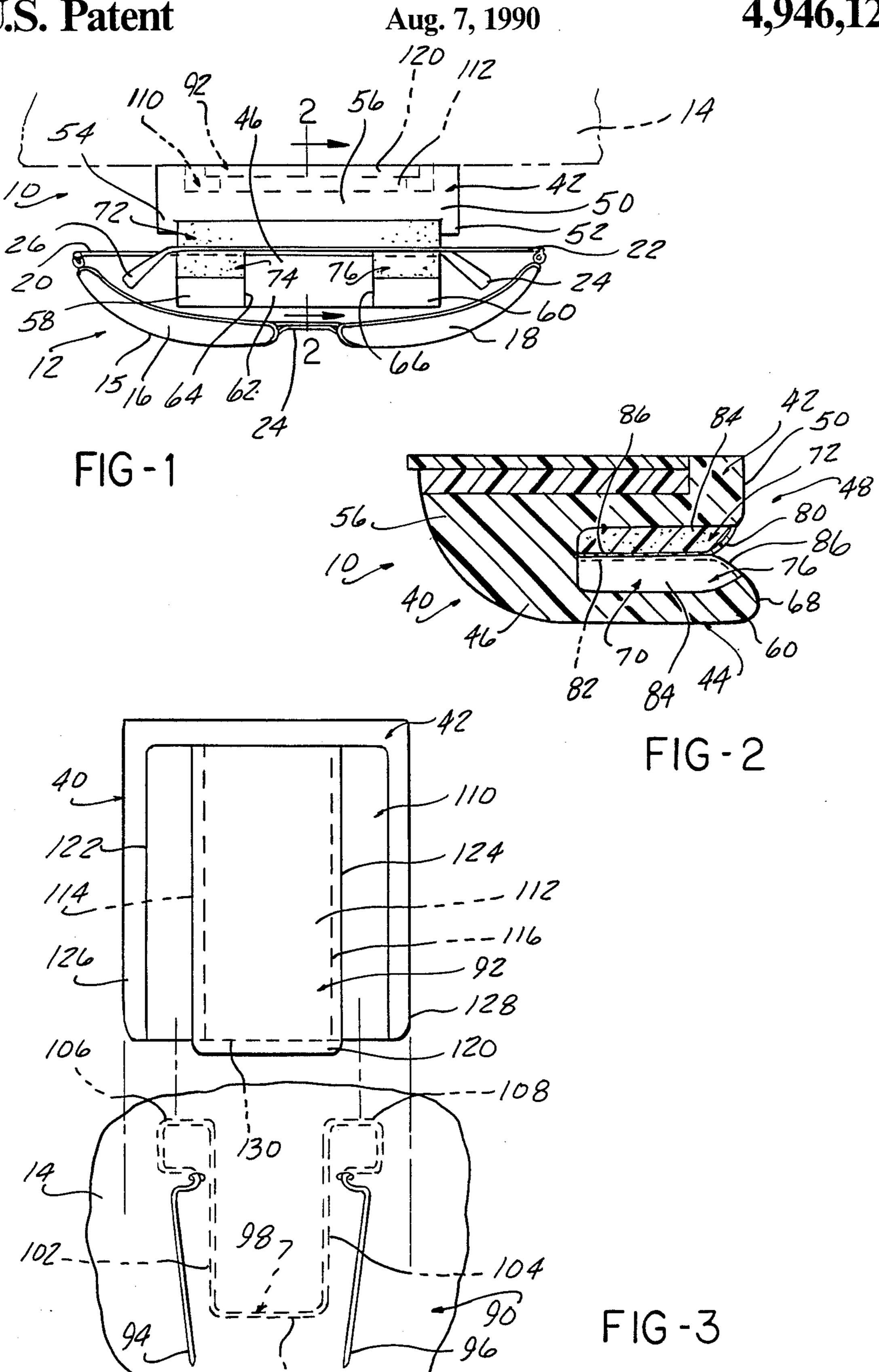
surface. Particularly, the present invention is an eyeglass holder mountable on a support surface within a vehicle, such as an automobile.
