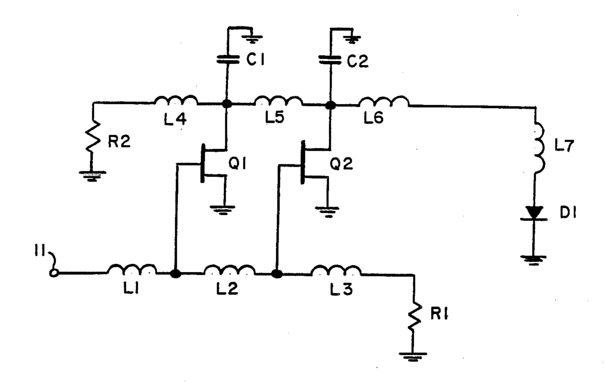
diode to be modulated is then connected to the low impedance end of the output circuit.
