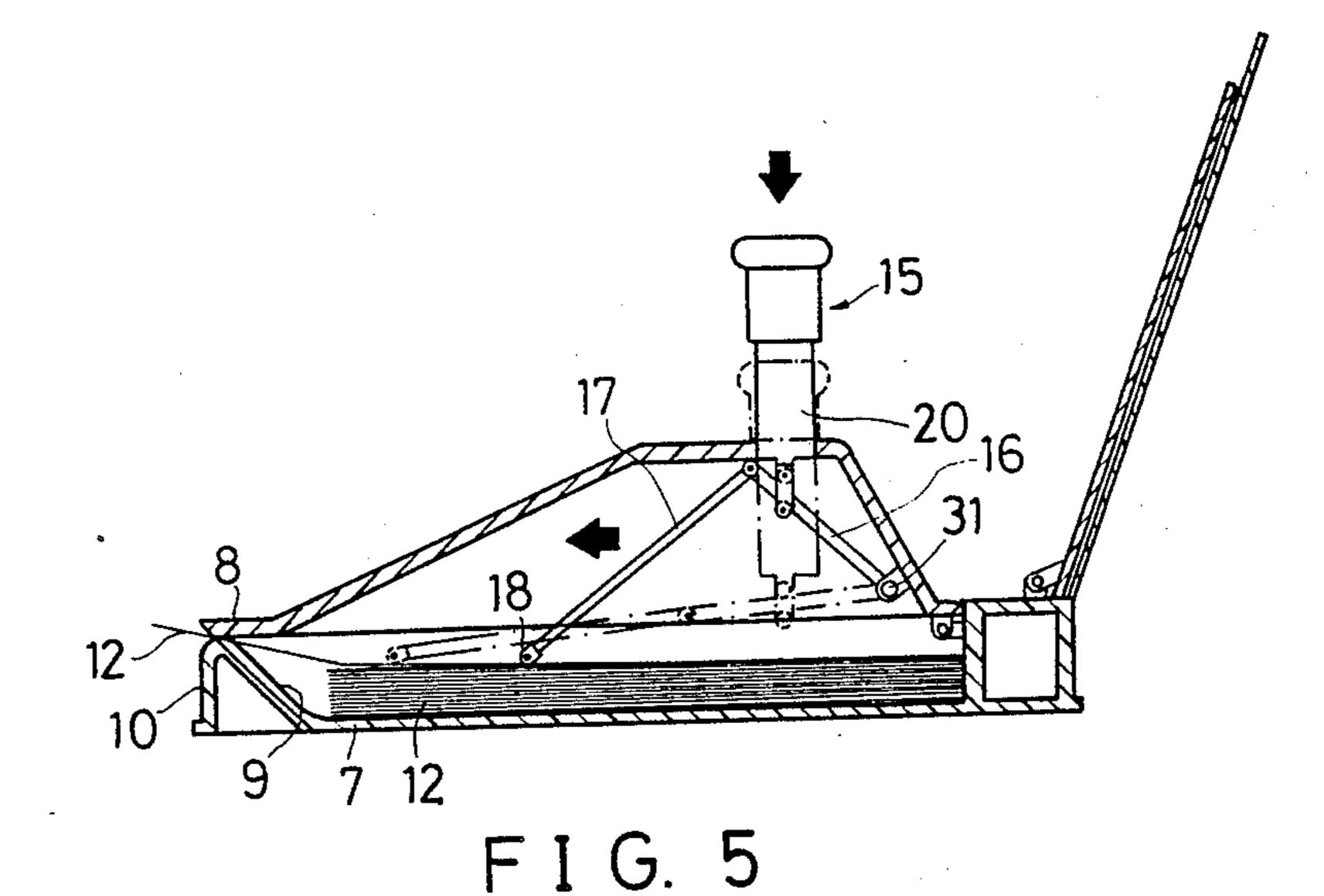
paper into the paper holder seat, through its fronted transparent or enlarged-functioned cover and the writing content remains for instant reading at any moment.
