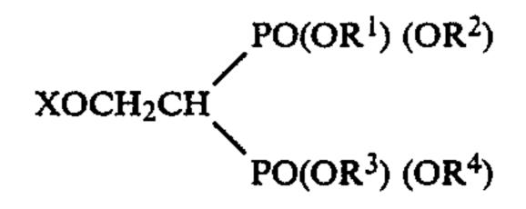
is formed by refluxing the above reactants in an alcohol solvent, such as ethanol or methanol, preferably methanol, typically at a temperature of from about 40° C. to about 80° C. Temperatures much below 40° C. do not provide effective conversion as the rate of reaction would be too slow. Temperatures of from about 55° C. to about 75° C. typically provide optimum conversion.
