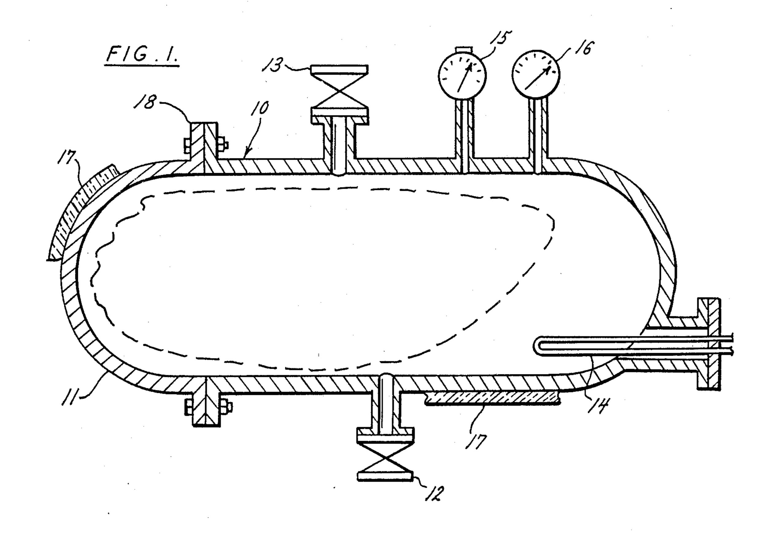
FILL VESSEL + HEAT WATER CHARGE PARTS WITH WATER CONTROL TEMPERATURE: 450 TO 500° REFILL WITH DRAIN VESSEL TIME: 1 TO 2 HOURS OLEIC ACID PRESSURE: 900 TO 1200 PSIG FLUSH PARTS DRAIN É TREAT PARTS WITH WATER WITH OLEIC ACID OPEN VESSEL RECOVER CLEAN DRY PARTS PARTS
