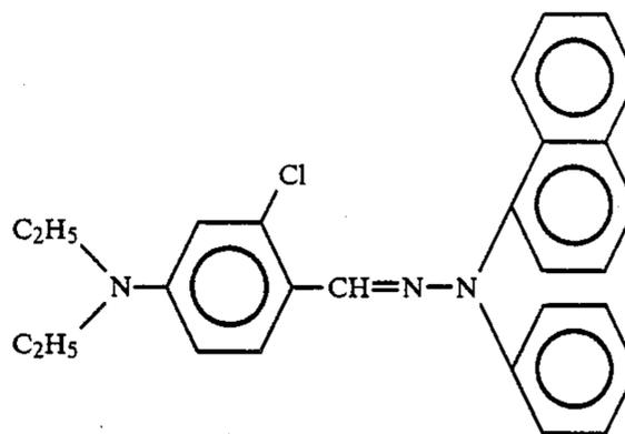
Further, one more photosensitive member was prepared in the same manner except for forming a charge transport layer with a composition comprising 8 parts of the hydrazone compound, 10 parts of the polycarbonate A and 4 parts of methaterphenyl (plasticizer).
