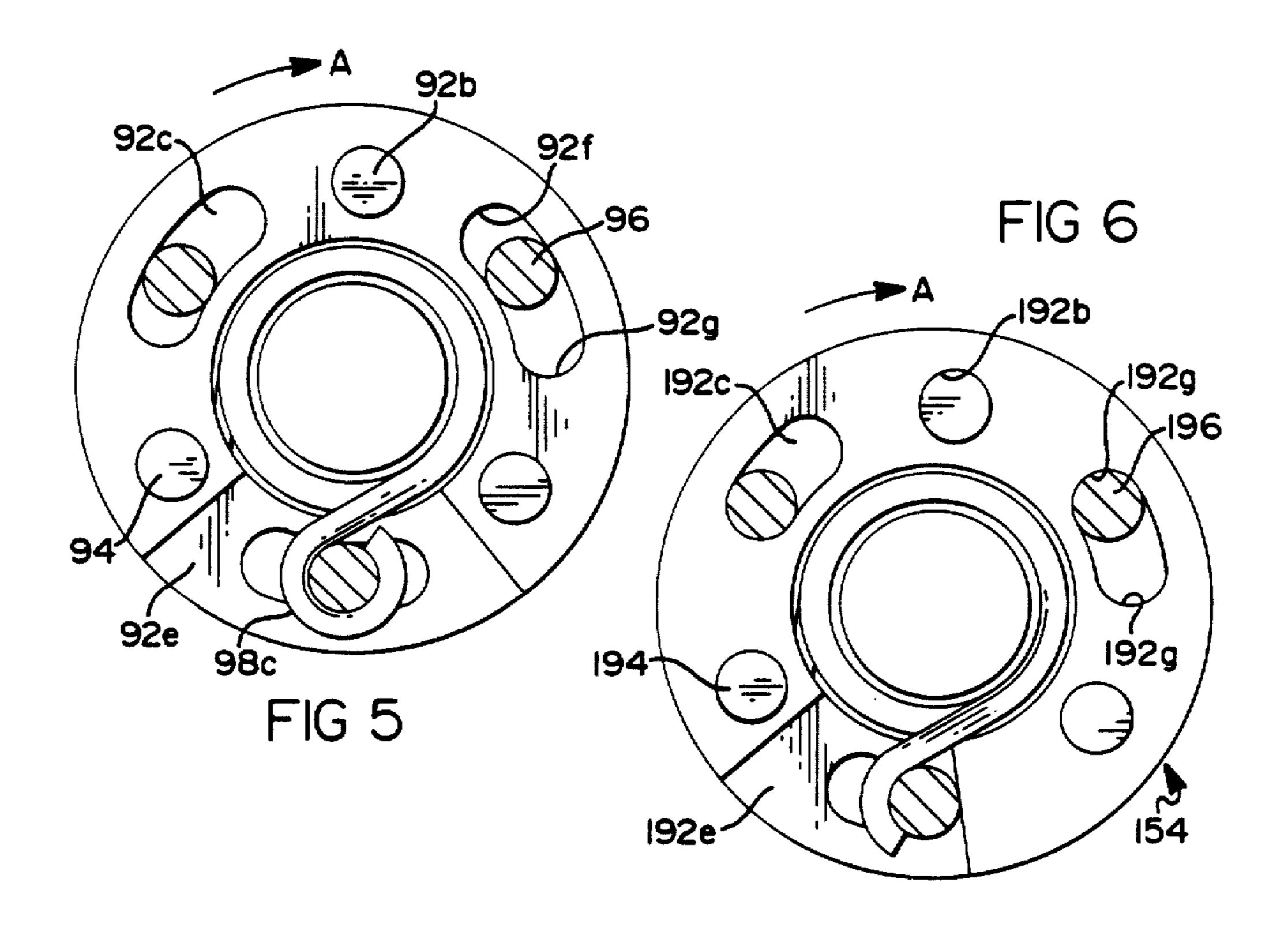
FIG. 6 is a detailed view of an alternative embodiment of the damping mechanism in FIGS. 3-5.
