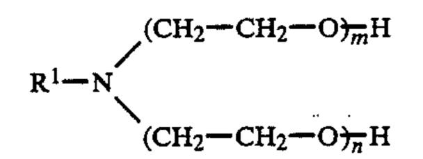
wherein R is alkyl or alkenyl each having 2 to 22 carbon atoms and the sum of m and n is a number from 2 to 30 is used as an improved biocide to preserve and protect aqueous solutions from infestation with micro-organisms.
