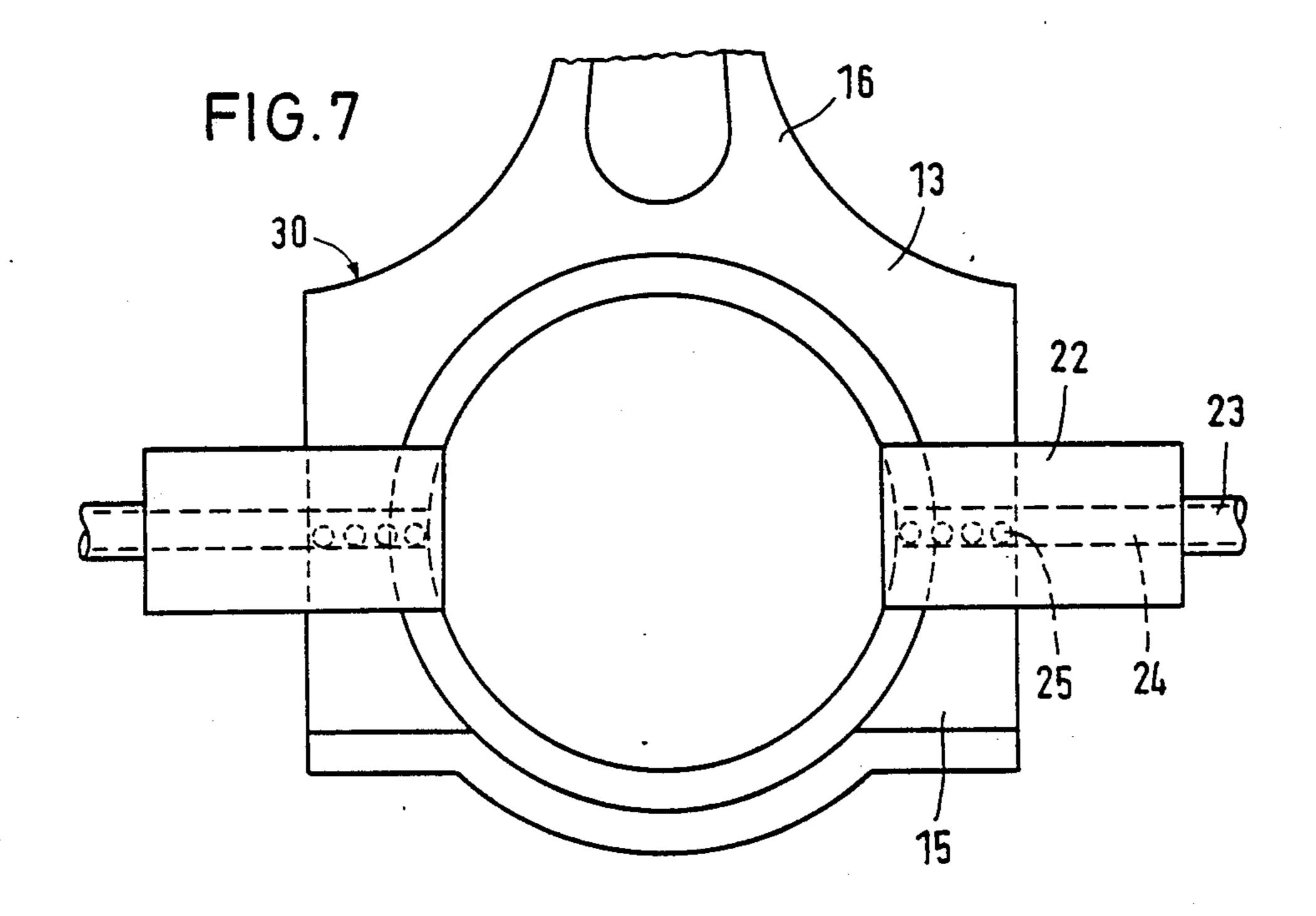
providing a protective layer on each tear notch; forging the preform into a component, including closing each tear notch during the forging to form a corre-
