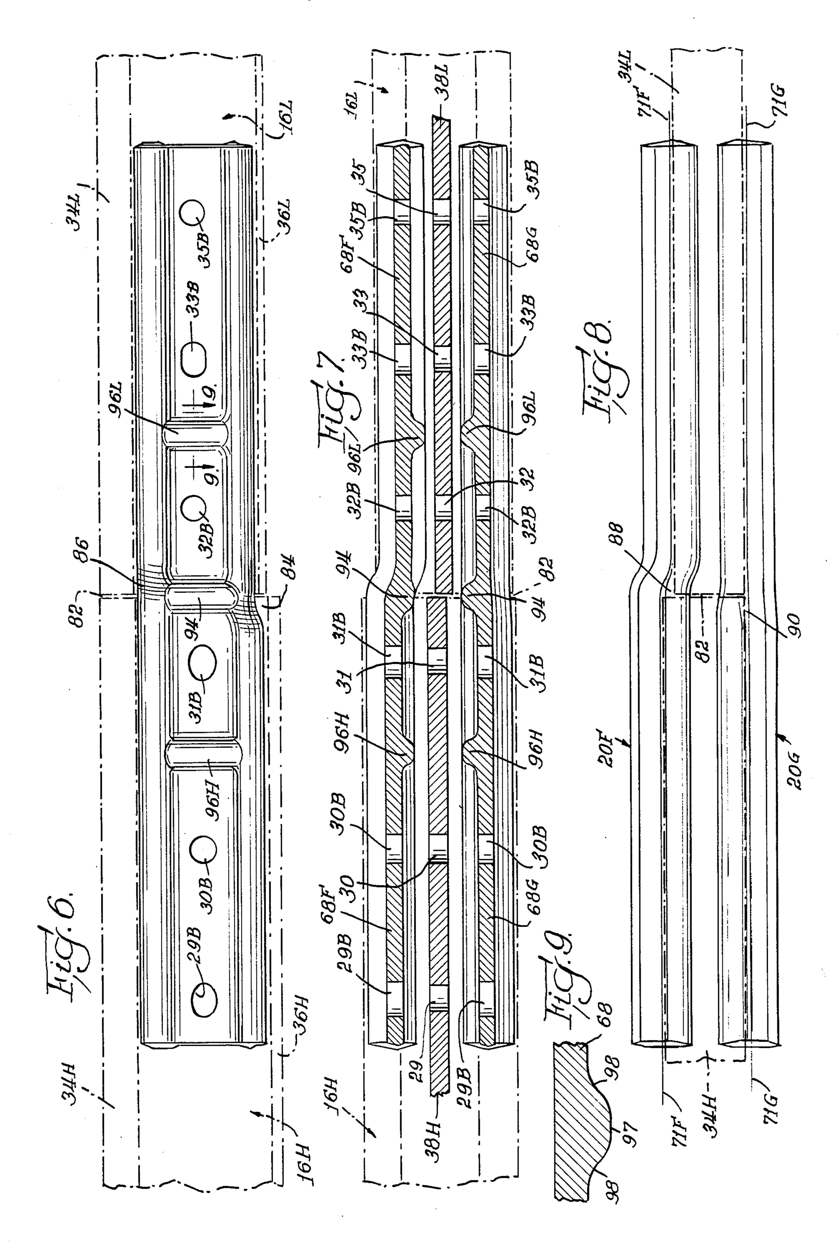
BAR FOR CONNECTING RAILWAY TRACK RAILS AND METHOD OF MAKING SAME
