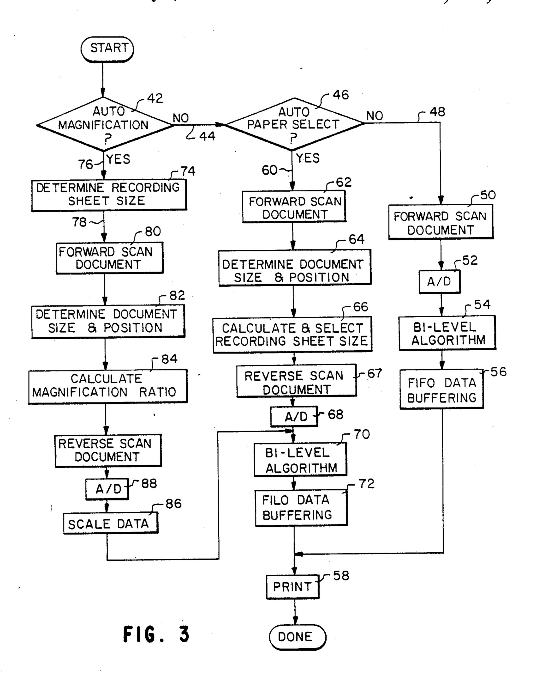
DOCUMENT RECOGNITION WITH FORWARD DIRECTION SCAN FOR DETECTING THE BOUNDARIES OF AN ORIGINAL DOCUMENT AND REVERSE DIRECTION SCAN FOR PRODUCING RECORDED IMAGE ON THE ORIGINAL DOCUMENT
