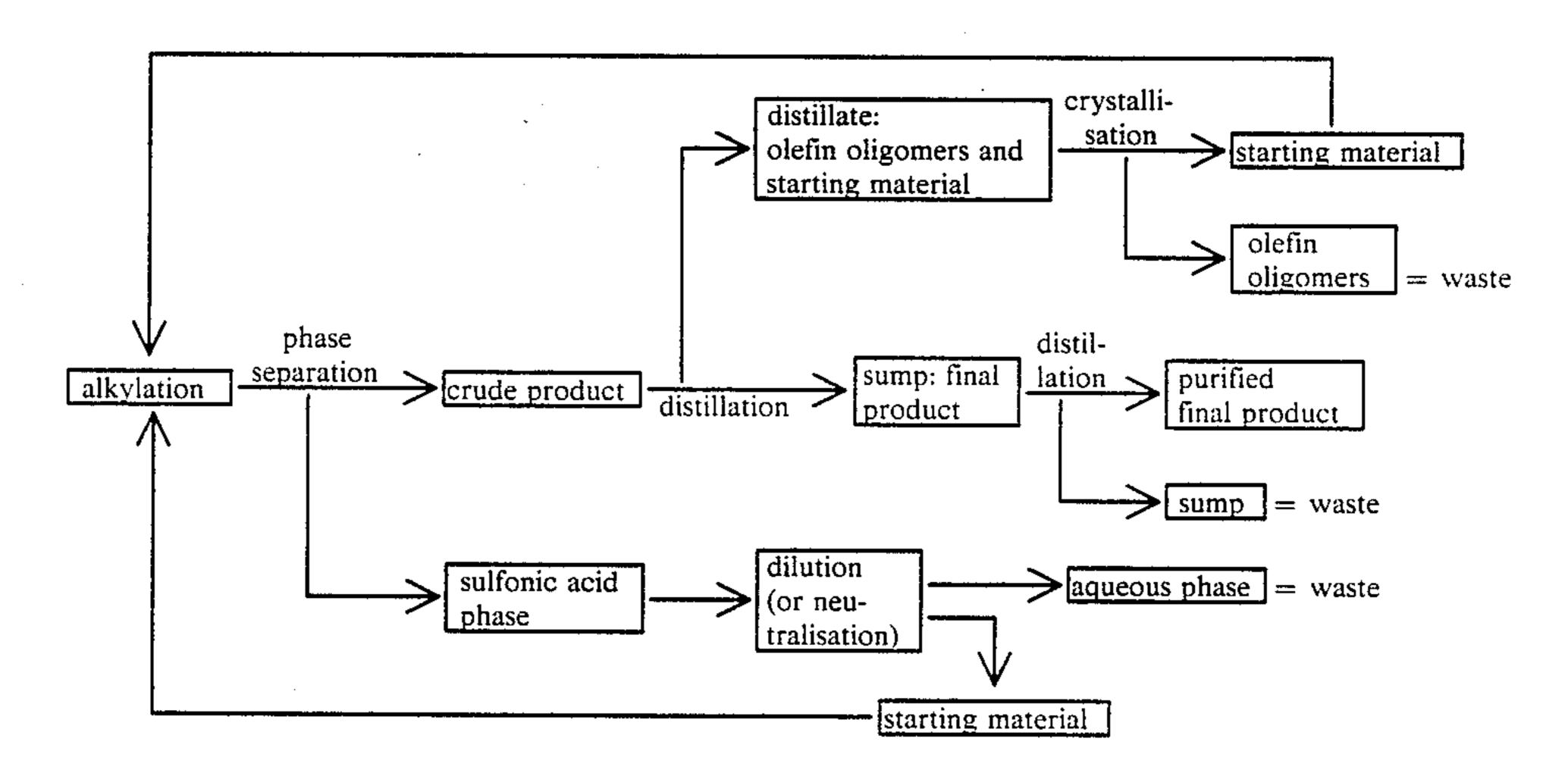
starting material = 2-(2-hydroxy-5-methylphenyl)benzotriazole final product = mixture of isomers of compounds of formula I
