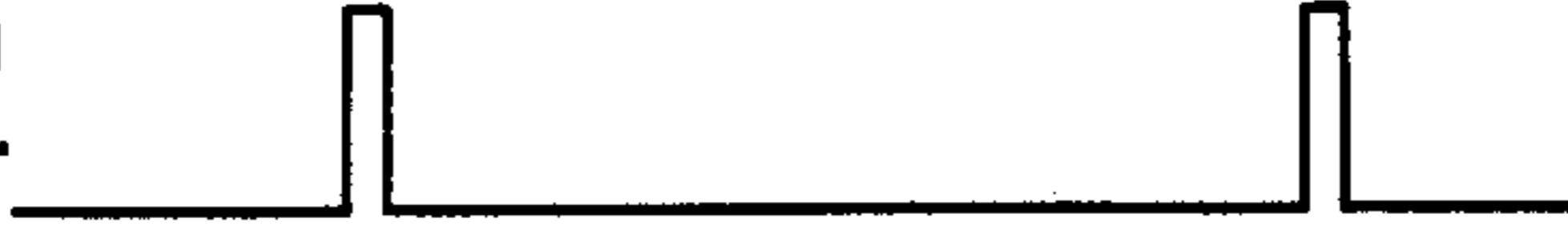
FIG. 9d OUTPUT TG1 OF AND CC.
