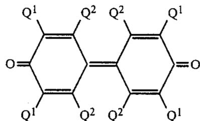
In many polyphenylene ethers obtained under the conditions described above, a substantial proportion of the polymer molecules, usually as much as about 90% by weight of the polymer, contain end groups having one or frequently both of formulas II and III. It should be understood, however, that other end groups may be present and that the invention in its broadest sense may not be dependent on the molecular structures of the polyphenylene ether end groups.
