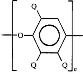
wherein the oxygen ether atom of one unit is connected to the benzene nucleus of the next adjoining unit,  $n$  is a positive integer and is at least 50, and each  $Q$  is a monovalent substituent selected from the group consisting of hydrogen, halogen, hydrocarbon radicals free of a tertiary alpha-carbon atom, halohydrocarbon radicals having at least two carbon atoms between the halogen atom and the phenyl nucleus, hydrocarboxy radicals, and the halohydrocarboxy radicals having at least two
