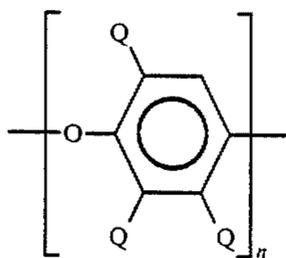
wherein the oxygen ether atom of one unit is connected to the benzene nucleus of the next adjoining unit,  $n$  is a positive integer and is at least 50, and each  $Q$  is a monovalent substituent selected from the group consisting of
