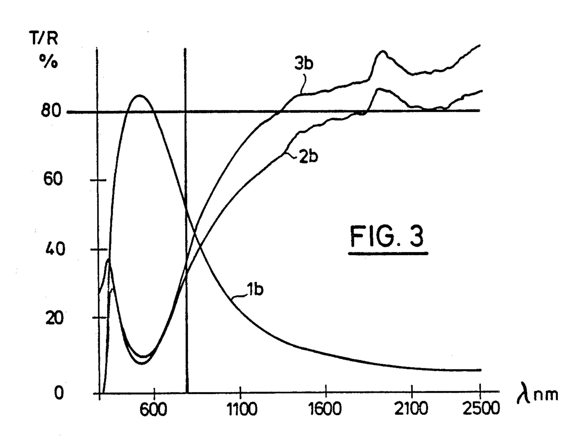
PROCESS FOR THE PRODUCTION OF CURVE GLAZING WITH A HIGH TRANSMITTANCE IN THE VISIBLE SPECTRAL RANGE AND A HIGH REFLECTANCE FOR THERMAL RADIATION
