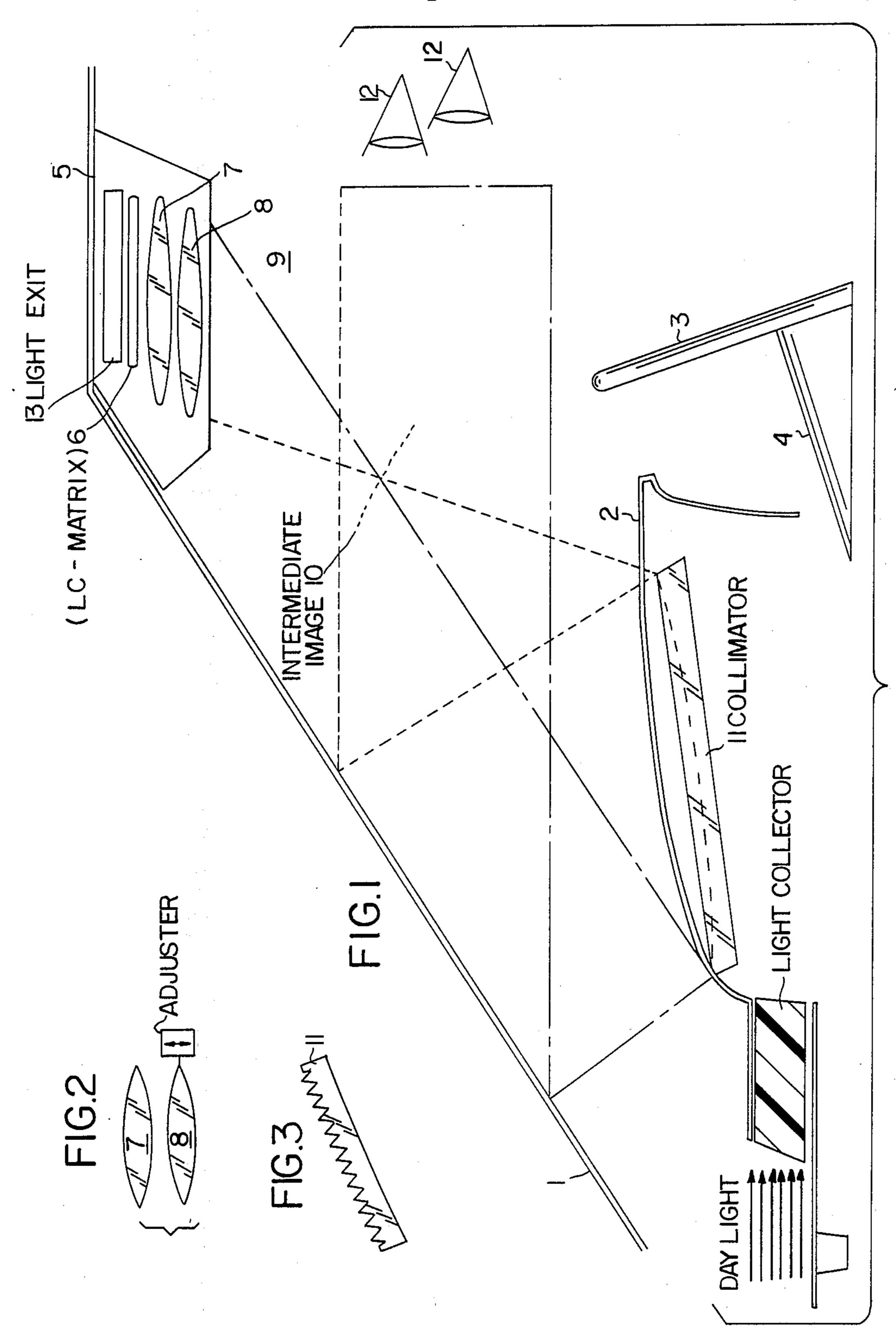
IMAGE-REPRODUCING ARRANGEMENT FOR MOTOR VEHICLES INCLUDING LENS MEANS FORMING A REAL IMAGE ADJACENT AN UPPER EDGE OF A WINDSHIELD TO WHICH AN INSTRUMENT PANEL MIRROR REFLECTS TO FORM A VIRTUAL IMAGE
