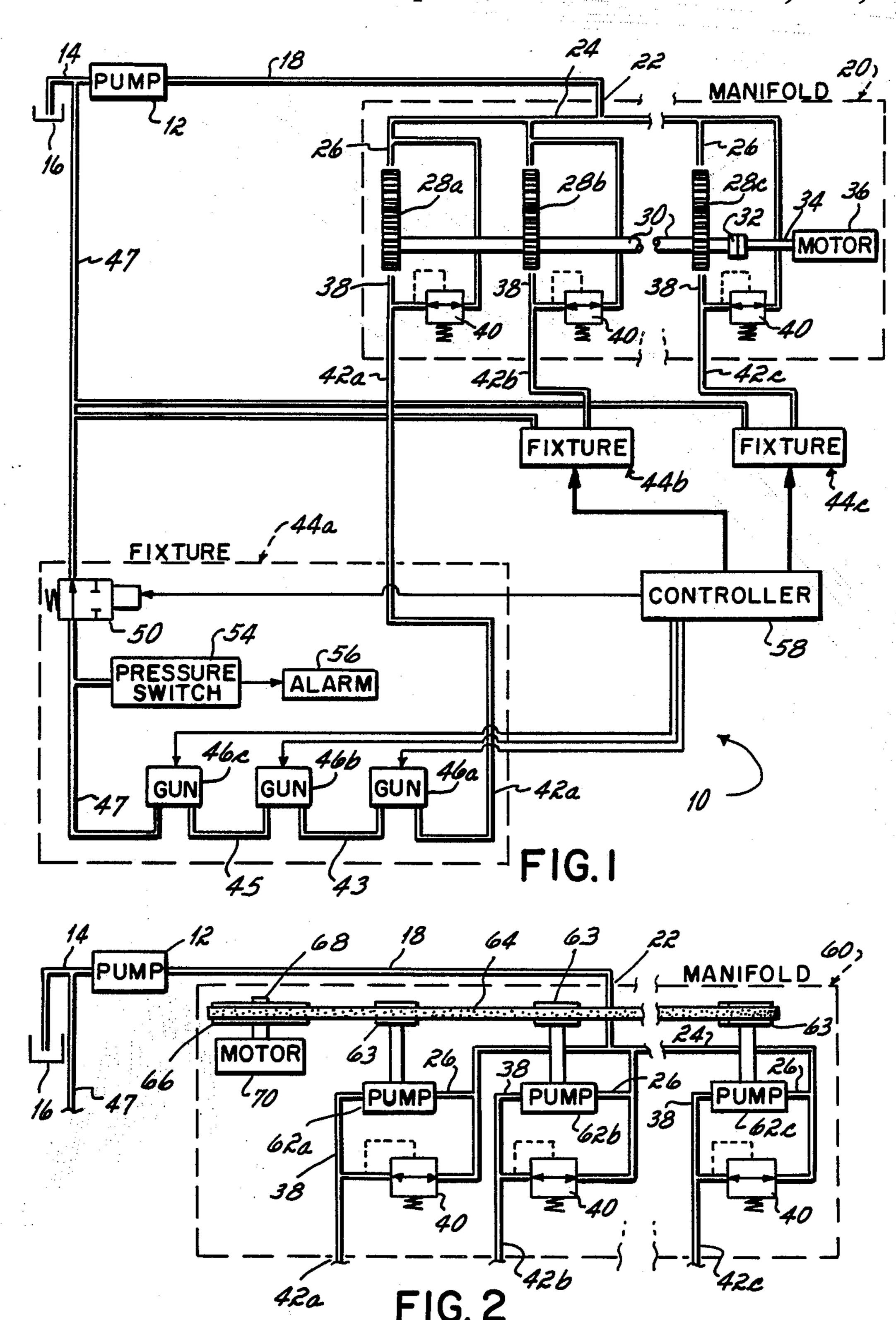
SPRAYING APPARATUS WITH FLOW ALARM
