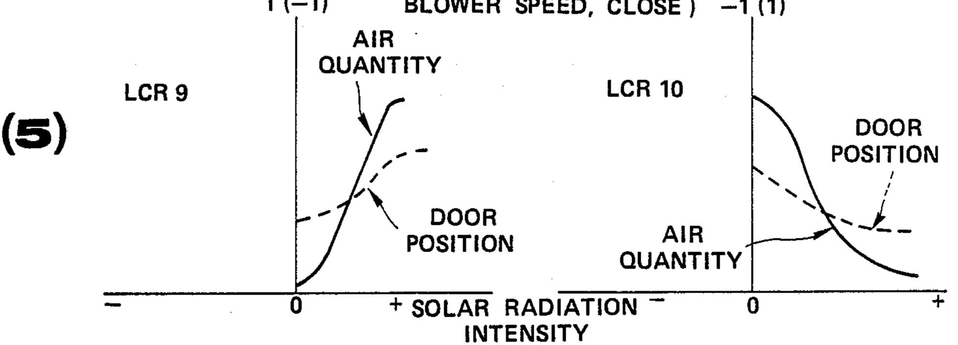
RELATION BETWEEN SOLAR RADIATION INTENSITY & AIR QUANTITY OR AIR MIX DOOR POSITION WHEN  $e>0\,(\,1\,\mbox{---}\,-\,$  HIGH BLOWER SPEED, OPEN ;
