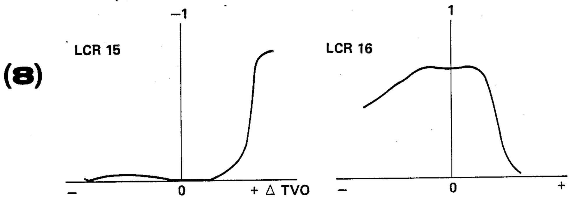
RELATION BETWEEN THROTTLE OPENING (TVO) & CLUTCH (1--- ENGAGE CLUTCH, -1--- DISENGAGE CLUTCH)
