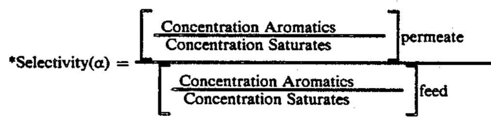
As can be seen from this table, it is not sufficient to meet just one of the recited criteria in order to obtain maximum selectivity. For instance, membranes in Examples 1 and 2 meet three of the criteria but because their functional groups are too far apart in the polymer (DF=6.5 and 5.5, respectively), the resulting flux is high and selectivity low. By increasing the Density
