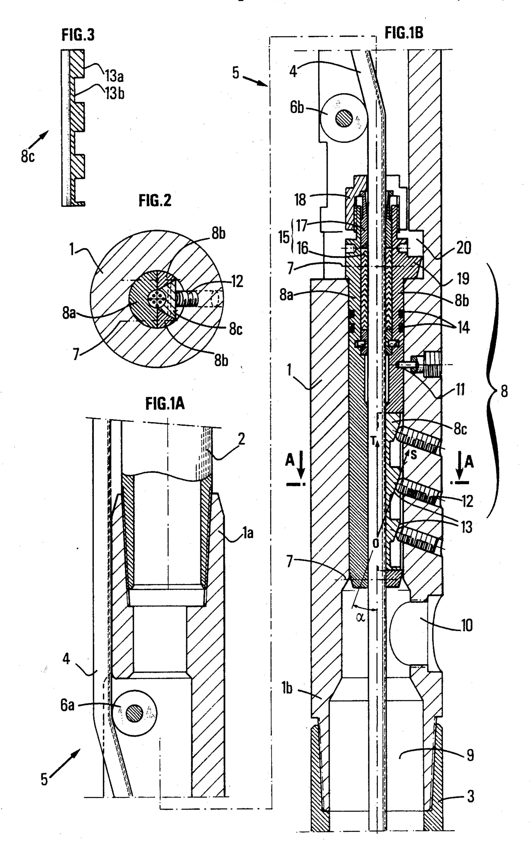
EQUIPMENT FOR A DRILL PIPE STRING INCLUDING A SIDE ENTRY SUB, A SAFETY MEMBER FOR ANCHORING A CABLE ON A SUPPORT, AND A METHOD OF USING THE EQUIPMENT
