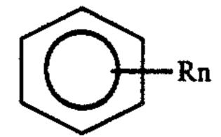
where R is methyl, ethyl, or a combination thereof, and n is an integer from 1 to 5. In other words, the aromatic substrate portion of the feedstock may be benzene, an 55 alkylaromatic containing from 1 to 5 methyl and/or ethyl group substituents, and mixtures thereof. Non-limiting examples of such feedstock compounds include benzene, toluene, xylene, ethylbenzene, mesitylene (1,3,5-trimethylbenzene) and mixtures thereof. It is spe-60 cifically preferred that the aromatic substrate is benzene.
