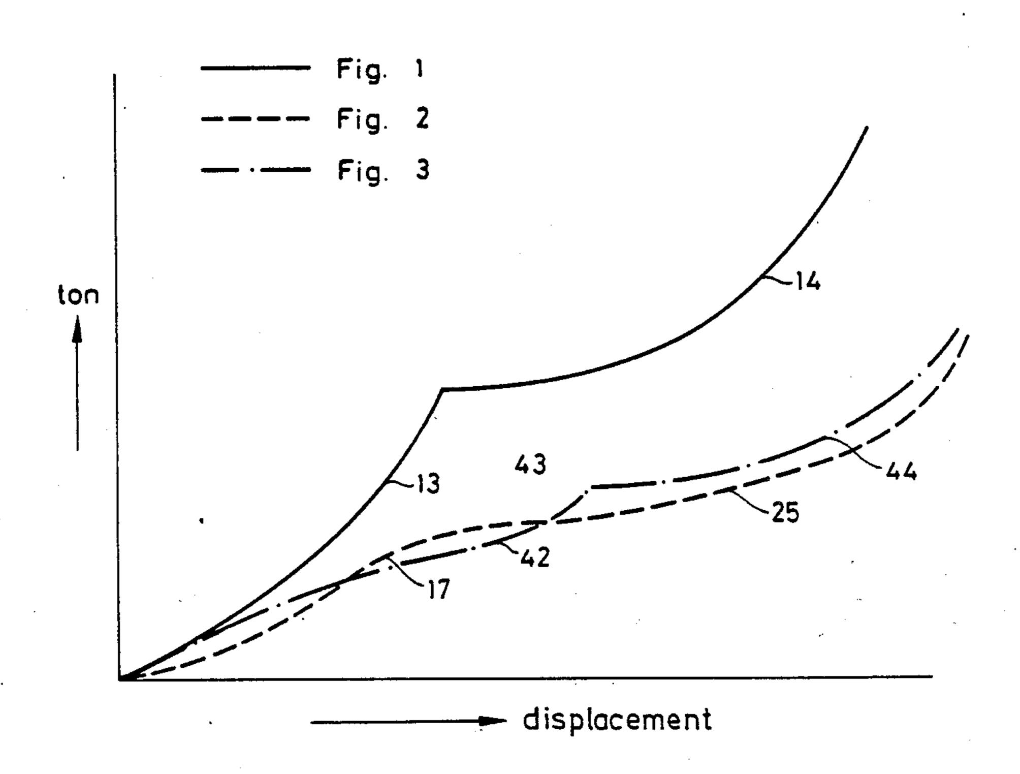
steep, the second spring will begin with an initially relatively flat curve, so that the increasing rigidity of the second spring does not take place until there is a
