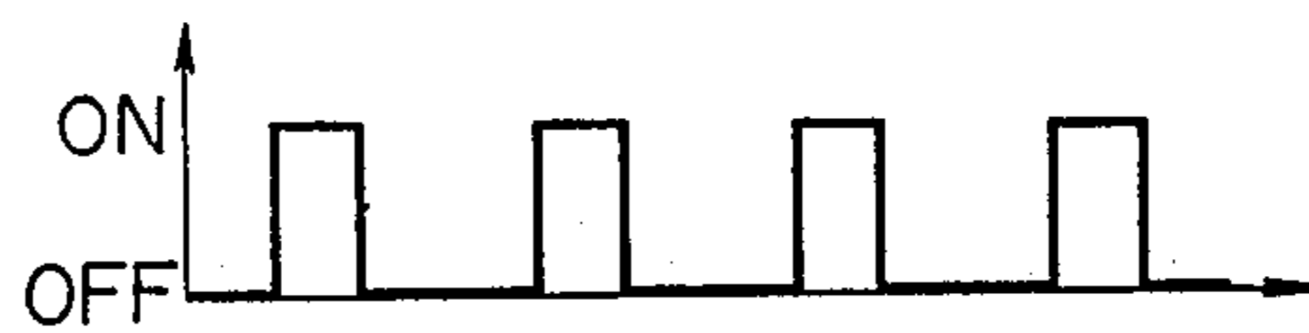
FIG. 15B(b) TRANSISTOR 15-5 CONTROL SIGNAL i_{TR}
