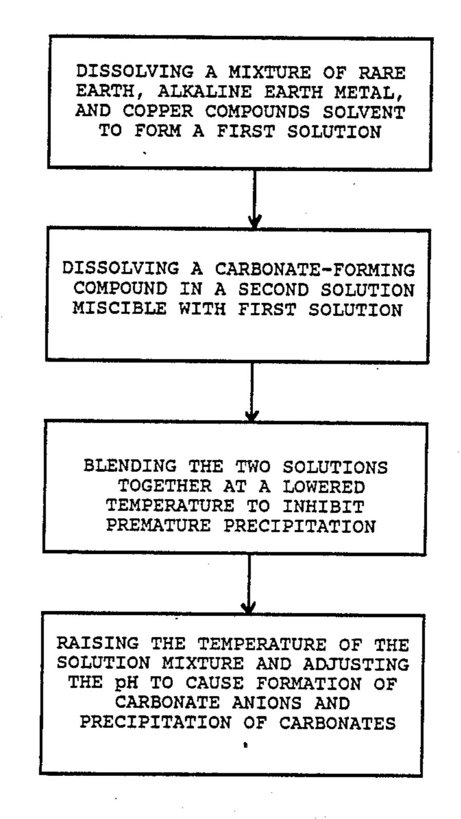
DISSOLVING A MIXTURE OF RARE EARTH, ALKALINE EARTH METAL, AND COPPER COMPOUNDS SOLVENT TO FORM A FIRST SOLUTION
