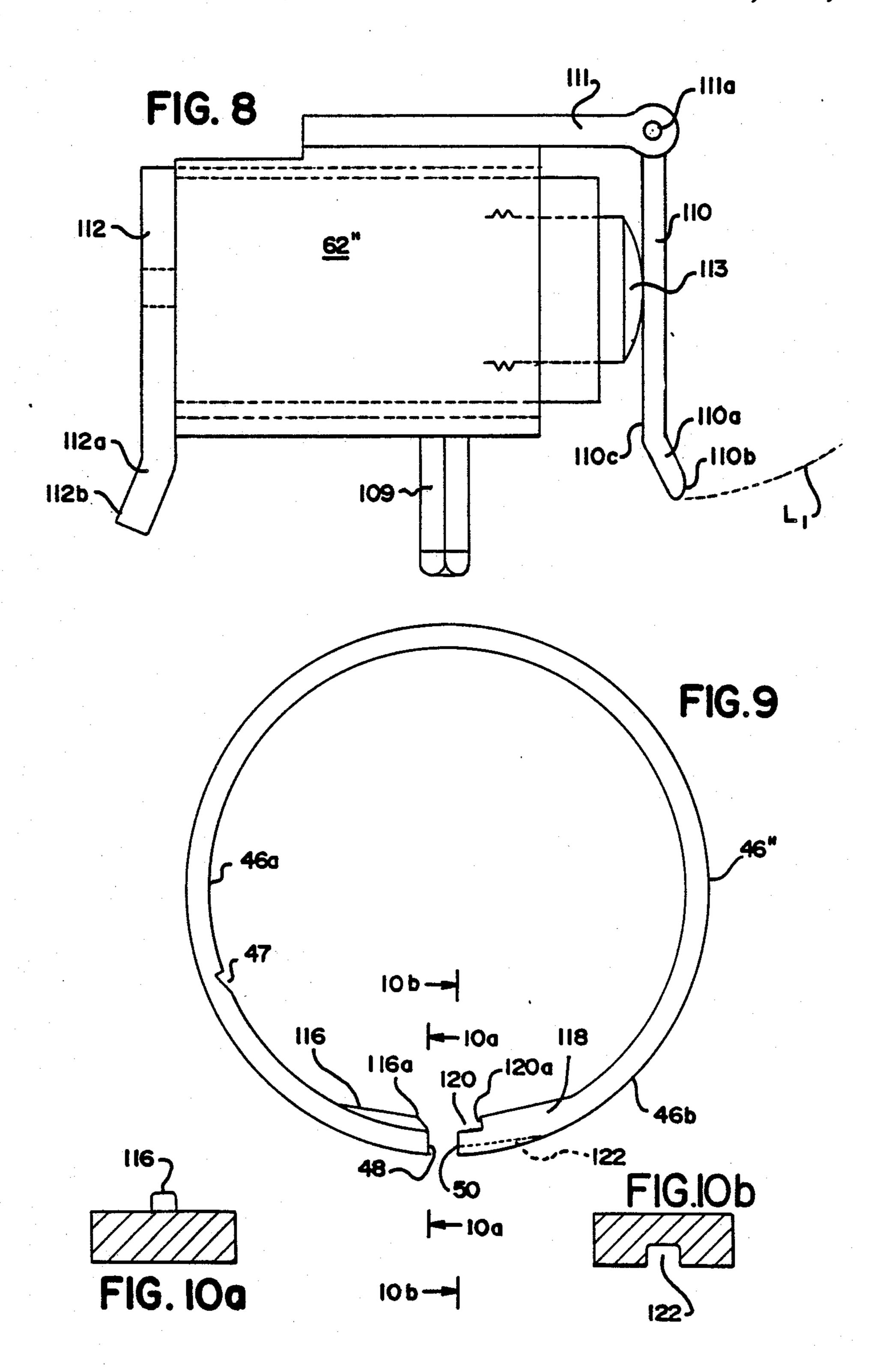
APPARATUS FOR PROVIDING A WATERTIGHT SEAL FOR MANHOLE PIPE CONNECTIONS INCLUDING A FOLDABLE GASKET AND CLAMPING BAND ASSEMBLY AND EXPANSION MEANS FOR INSTALLING THE GASKET AND CLAMPING BAND ASSEMBLY
