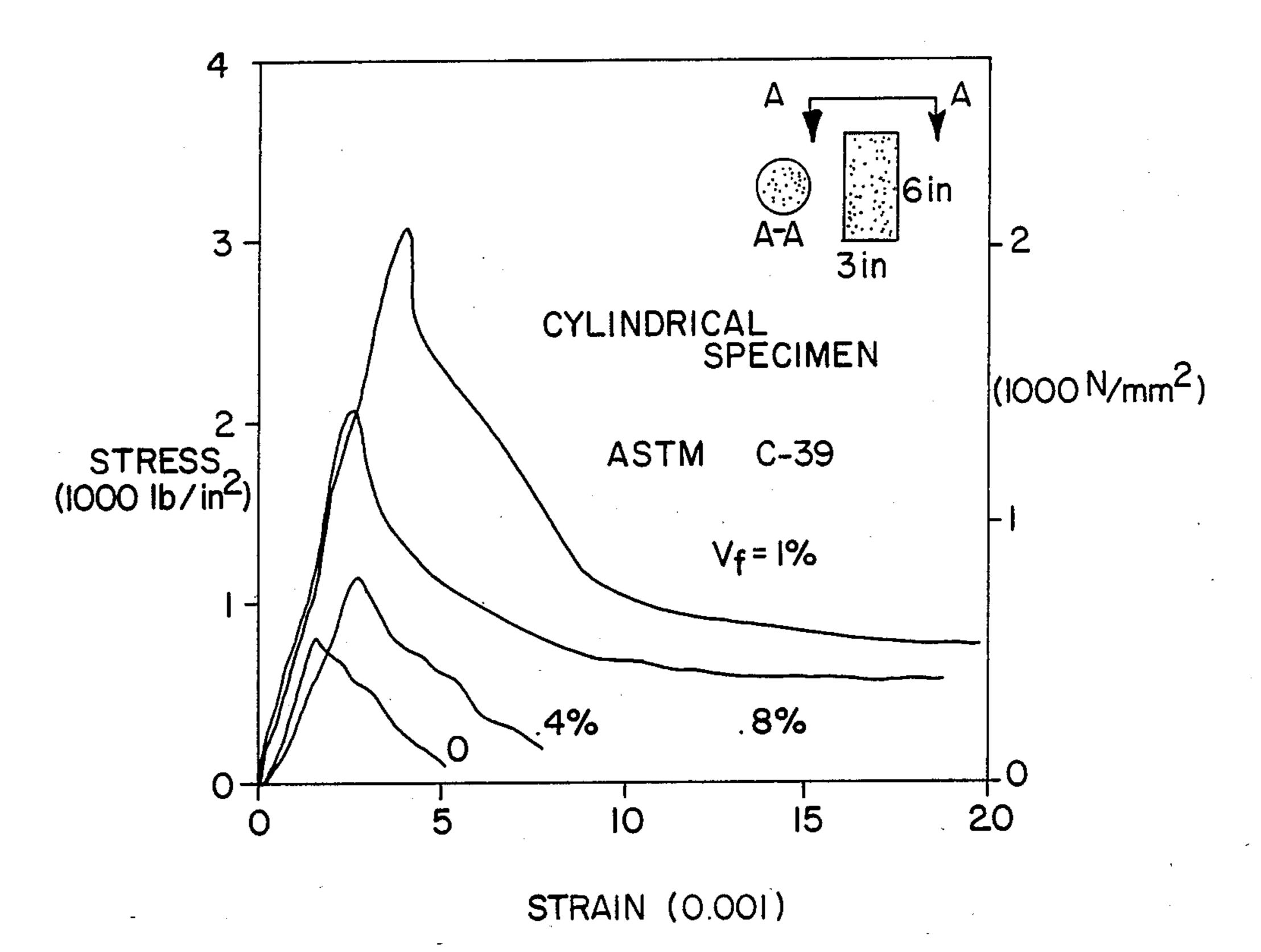
V<sub>f</sub>=FIBER VOLUME FRACTION FIBER LENGTH = .5in(12.7 mm)
