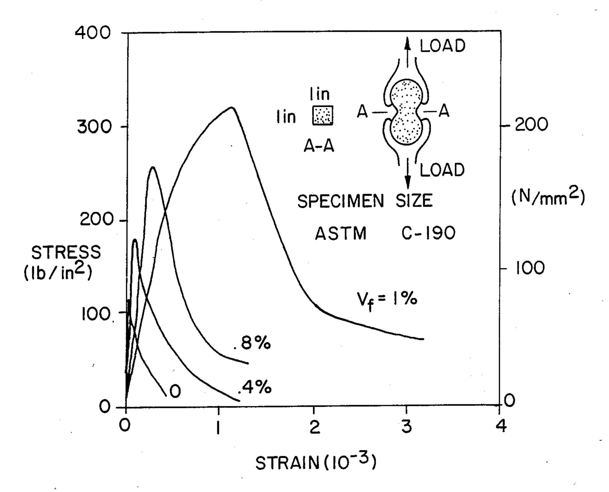
$V_f$  = FIBER VOLUME FRACTION FIBER LENGTH = .5in (12.7 mm)
