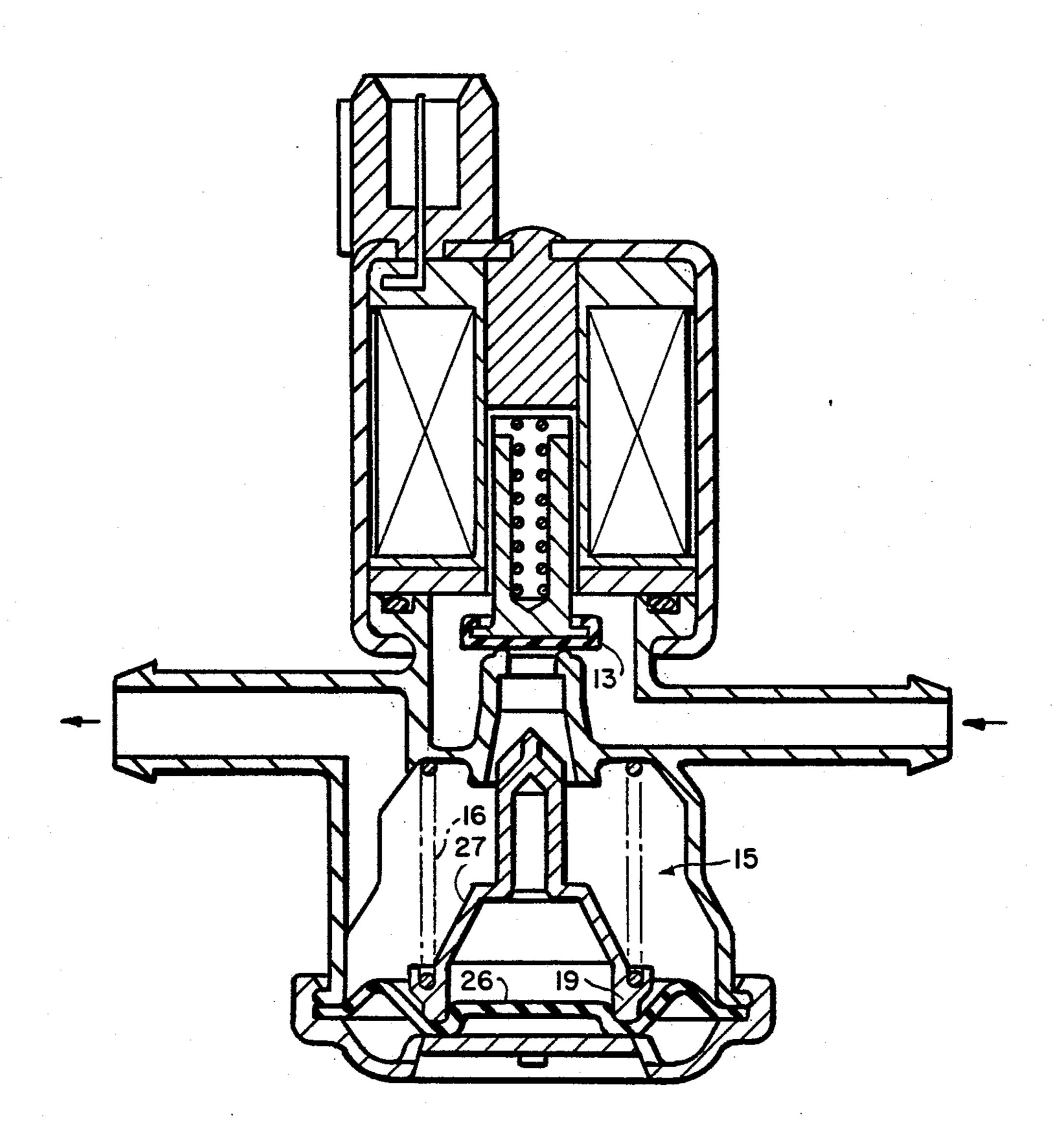
APPARATUS FOR THE MEASURED FEEDING OF **VOLATILE FUEL COMPONENTS TO THE** INTAKE TUBE OF AN INTERNAL COMBUSTION ENGINE
