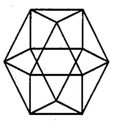
This twelve-cornered polyhedron structure is the metal atom configuration of a typical HPA described above. Between any two metal atoms is an oxygen atom, not shown, and from each metal atom is a doubly bonded oxygen, also not shown, and each of the metal atoms is bonded through oxygen to the central metal atom, not shown.
